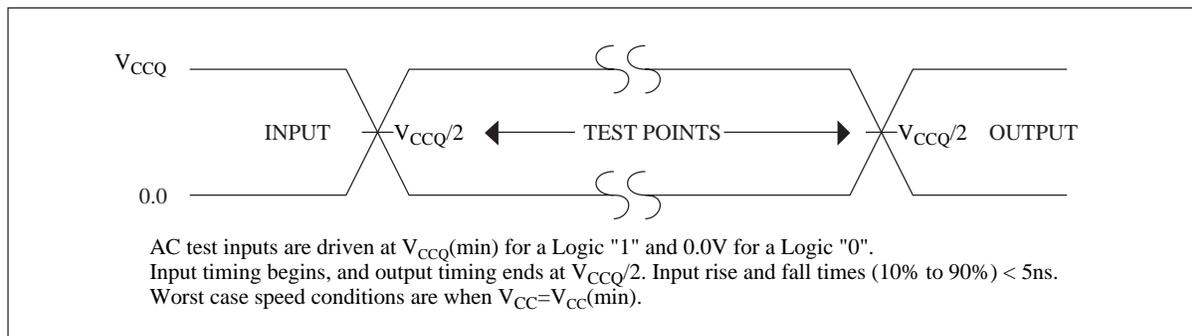
Figure 4. Transient Input/Output Reference Waveform for  $V_{CC}=2.7\text{V}-3.6\text{V}$
