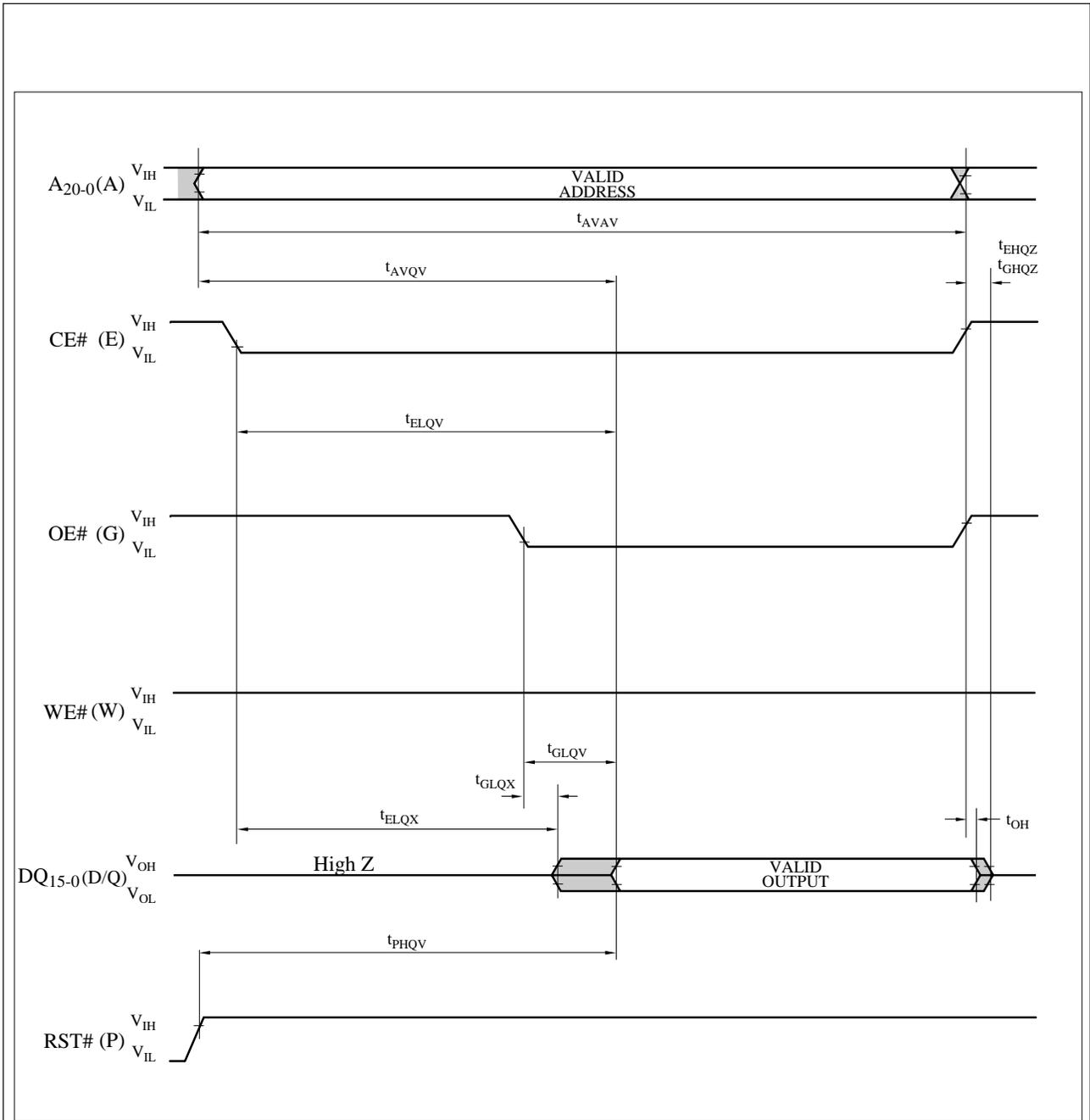
Figure 6. AC Waveform for Read Operations
