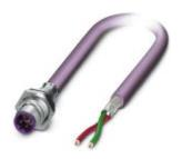
Bus system flush-type plug, PROFIBUS, 2-pos., M12, shielded, B-coded, SPEEDCON, rear/screw mounting with Pg9 thread, with 1.0 m bus cable,  $2 \times 0.25 \text{ mm}^2$
