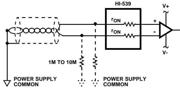
NOTE: The amplifier in Figure 8A is unusable because its bias currents cannot return to the power supply. Figure 8B shows two alternative paths for these bias currents: either a pair of resistors, or (better) a third wire from the low side of the signal source.
