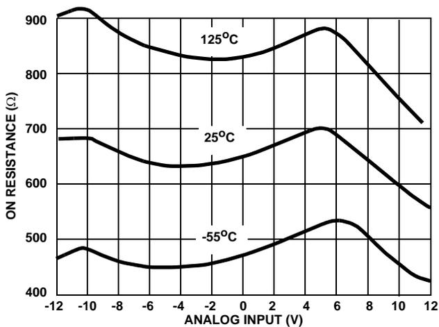
FIGURE 1C. ON RESISTANCE vs ANALOG INPUT VOLTAGE
