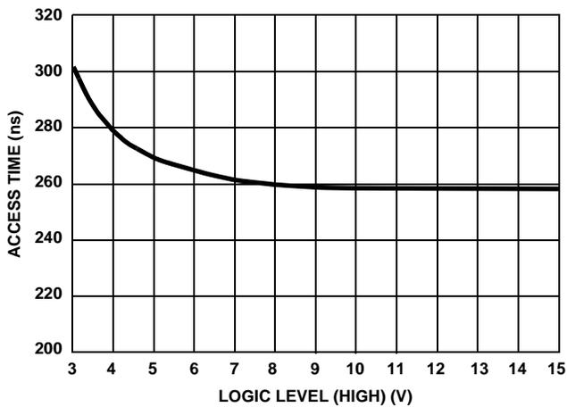
FIGURE 4A. ACCESS TIME vs LOGIC LEVEL (HIGH)
