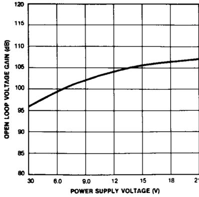
Figure 1. Open-Loop Voltage Gain vs Power Supply Voltages
