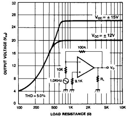
Figure 4. Output Voltage Swing vs Load Resistance
