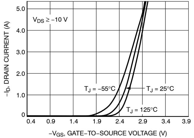
Figure 2. Transfer Characteristics
