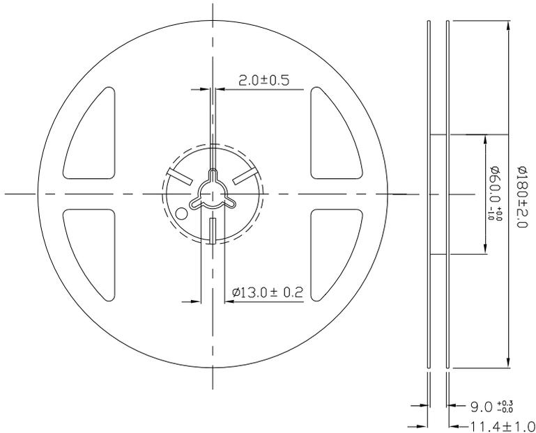
**Carrier Tape Dimensions: Loaded quantity 3000 PCS per reel**
