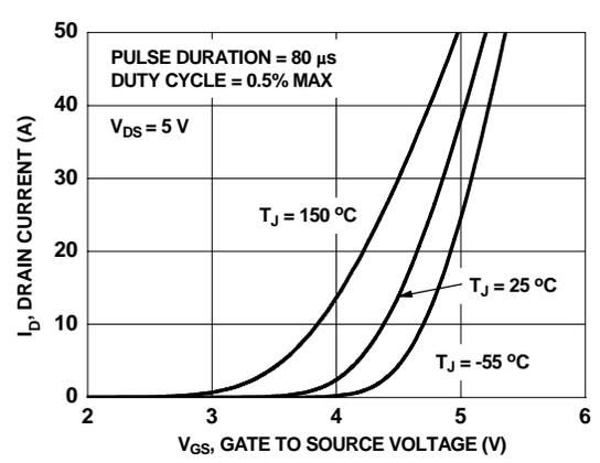
**Figure 5. Transfer Characteristics**
