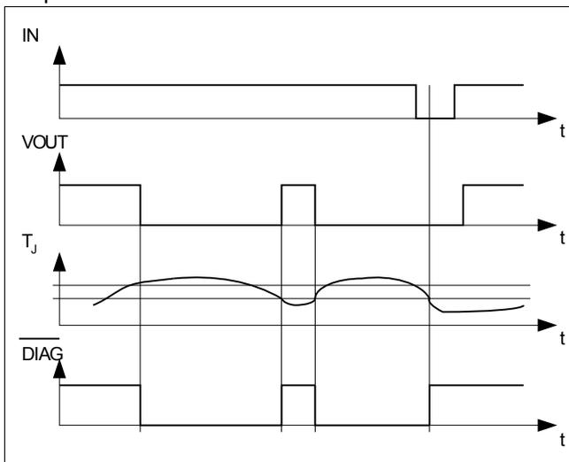
**Figure 5 Overtemperature detection**
