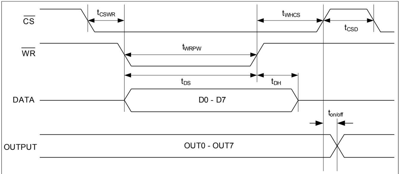
**Figure 11** Parallel input - output timing diagram
