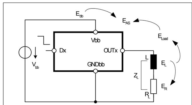
**Figure 4 Inductive load switch-off energy dissipation (each channel)**
