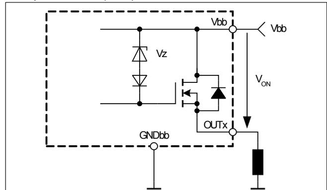
**Figure 3 Inductive and overvoltage output clamp (each channel)**
