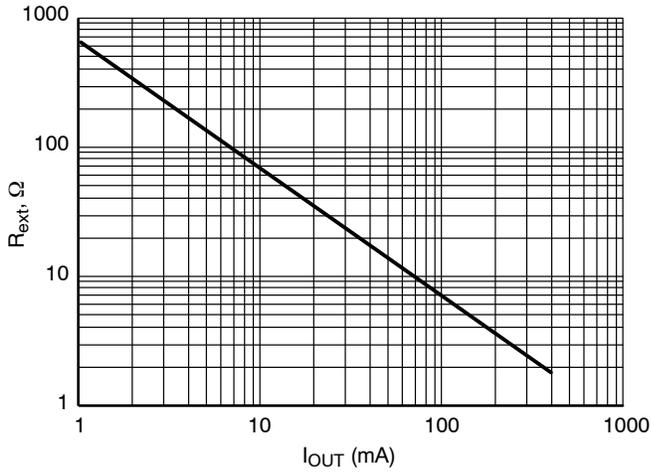
**Figure 1. Output Current ( $I_{OUT}$ ) vs. External Resistor ( $R_{ext}$ )**
