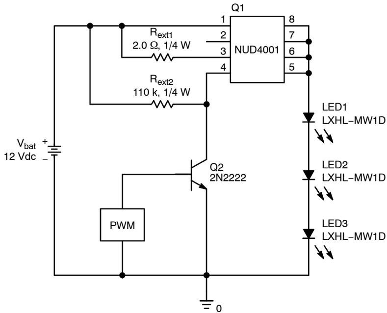
**Figure 9. NUD4001 Device Configuration for PWM**
