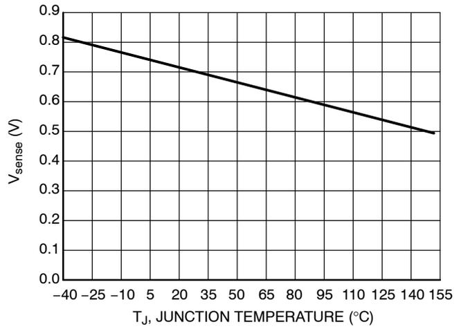
**Figure 2.  $V_{sense}$  vs. Junction Temperature**
