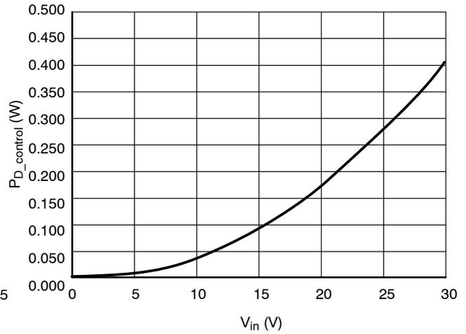
**Figure 4. Internal Circuit Power Dissipation vs. Input Voltage**
