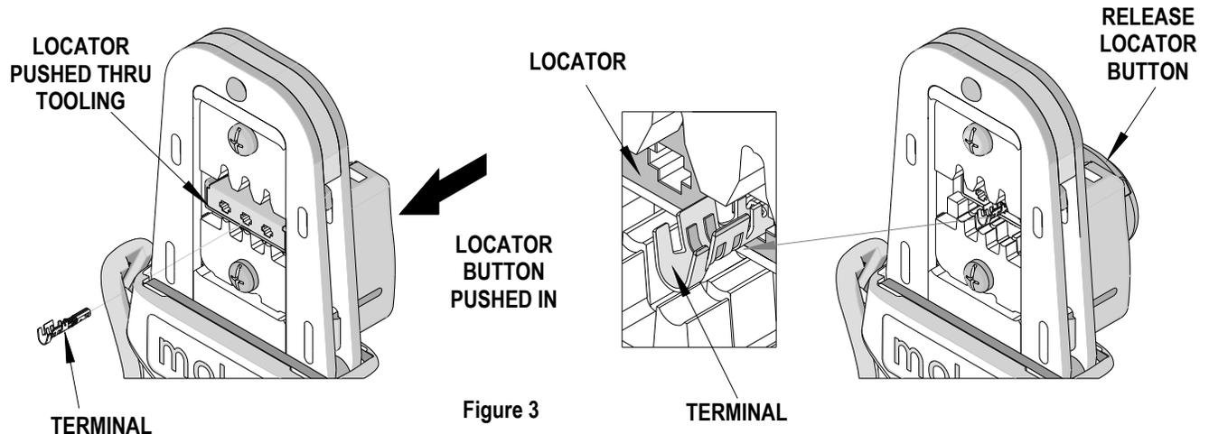
3. While holding the locator button in, load the terminal into the proper nest opening in the locator based on the wire gauge or terminal type markings on the hand tooling. See Figure 3.
