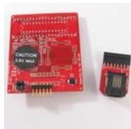
This Processor Extension Pak is designed for those who wish to debug with PIC16LF1907 family of microcontroller in-circuit. In addition to the debug capabilities available on the production variants of PIC16F1907 family, this Processor Extension Pak provides additional enhanced debug capabilities while freeing up I/O pins.
