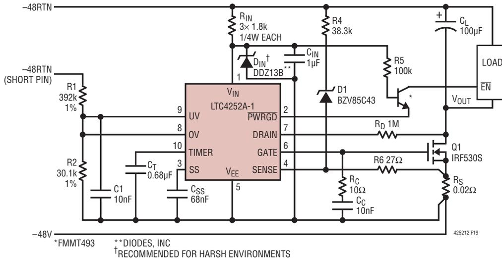
Figure 19. Power Limit Circuit Breaking Application
