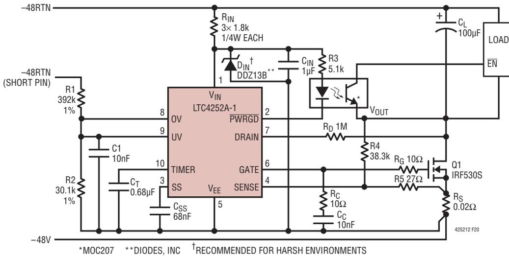
Figure 20. Circuit Breaker with Foldback Current Limit Application
