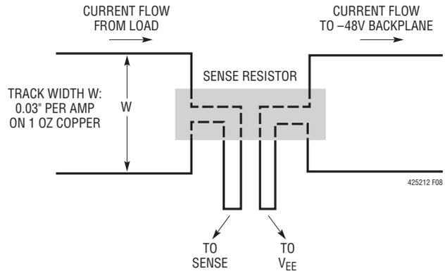
**Figure 8. Making PCB Connections to the Sense Resistor**
