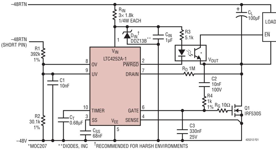
Figure 21. Inrush Control Without a Sense Resistor Application
