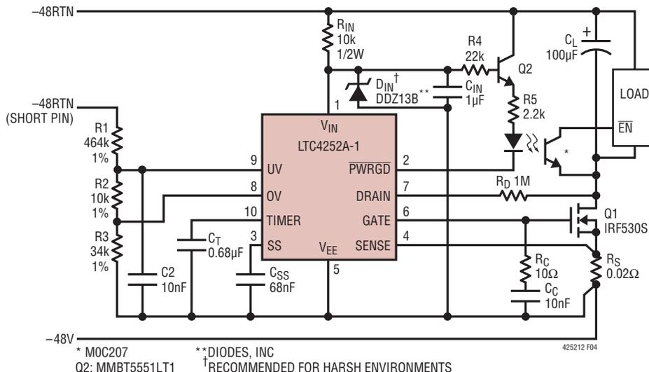
Figure 4. -48V/2.5A Application with Wider Input Operating Range
