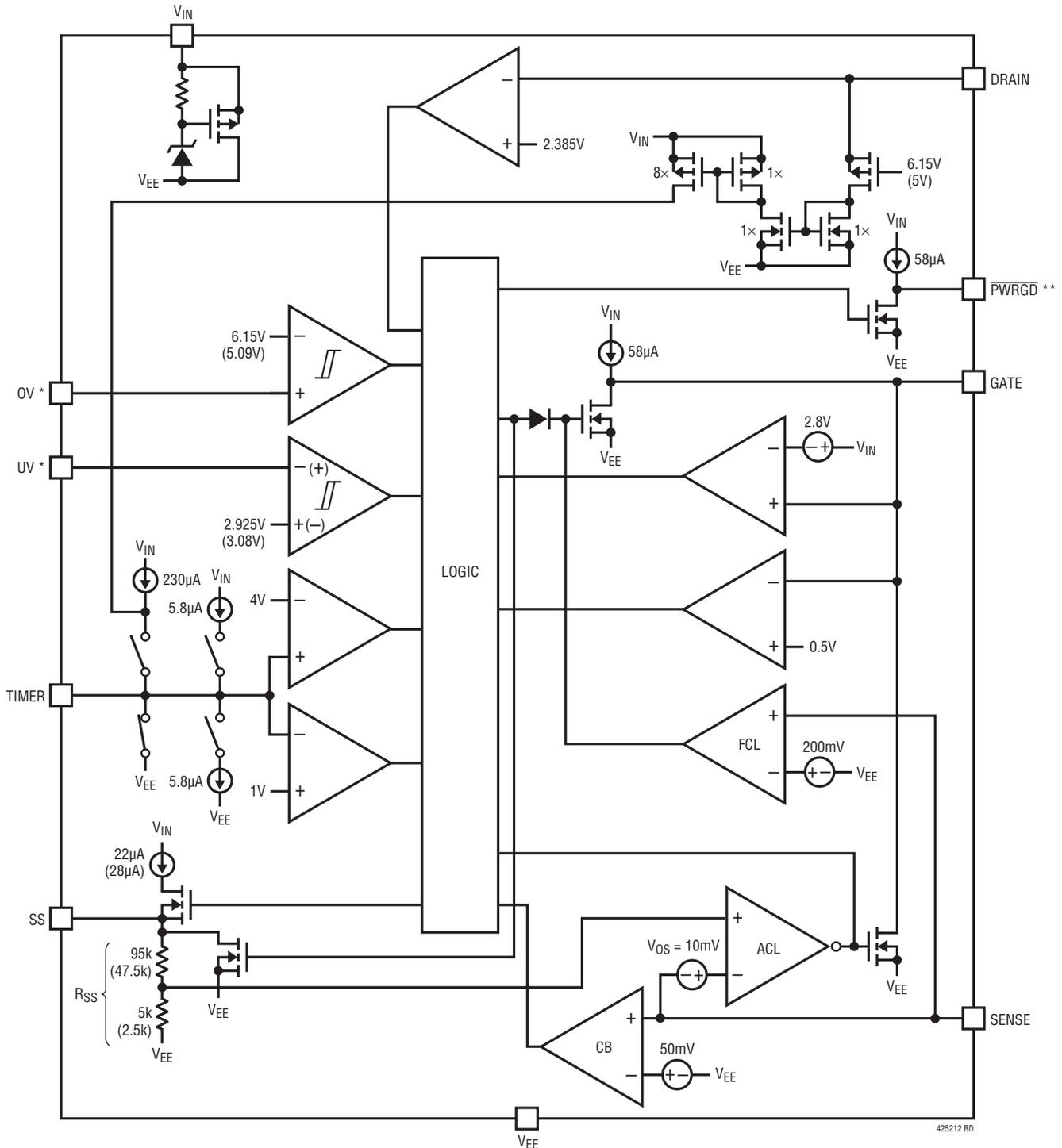
\*OV and UV ARE TIED TOGETHER ON THE MS8 PACKAGE. OV and UV ARE SEPARATE PINS ON THE MS PACKAGE
