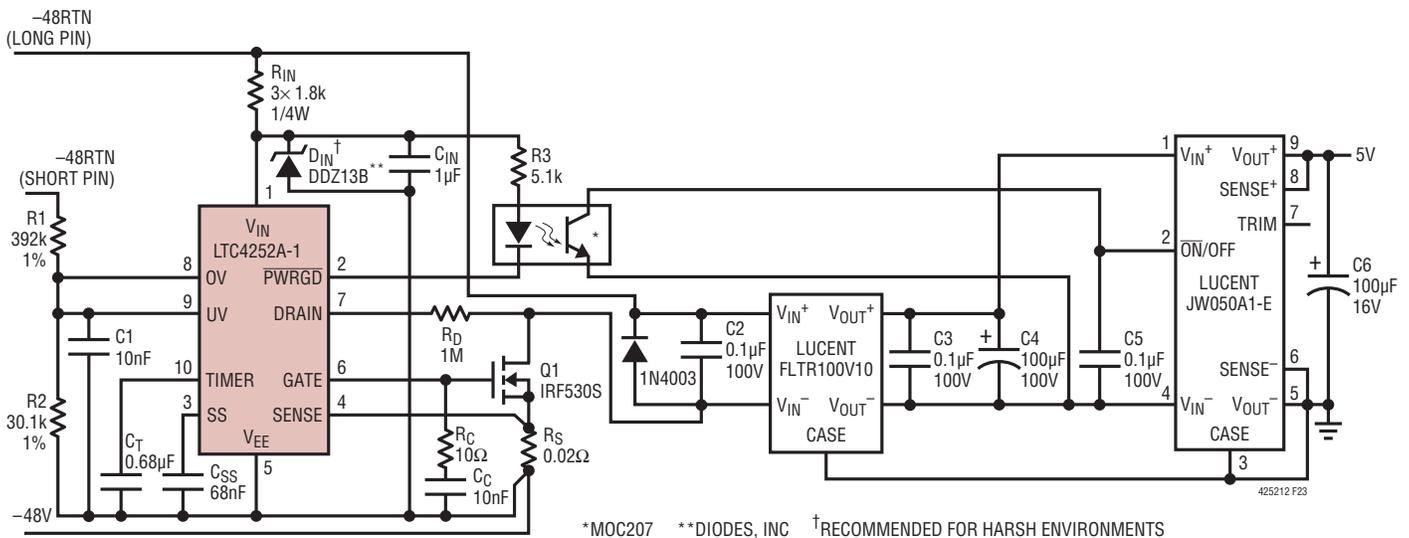
Figure 23. Typical Application Using a Filter Module
