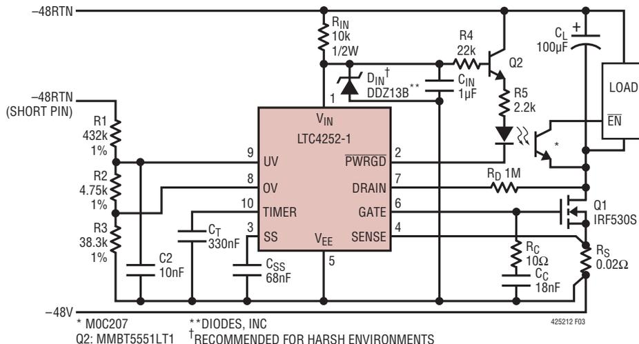
Figure 3.  $-48\text{V}/2.5\text{A}$  Application with Different Input Operating Range
