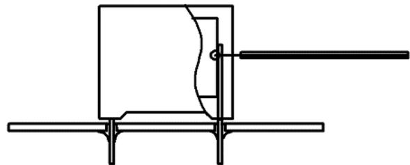
*Temperature monitored inside the capacitor.*
