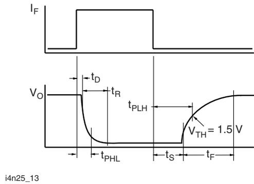
Fig. 13 - Switching Timing
