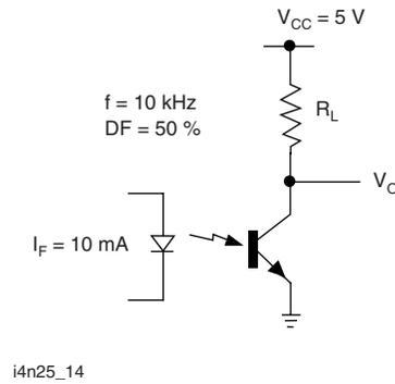
Fig. 14 - Switching Schematic
