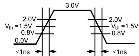
TTL Input Test Waveform (CY7B991)
