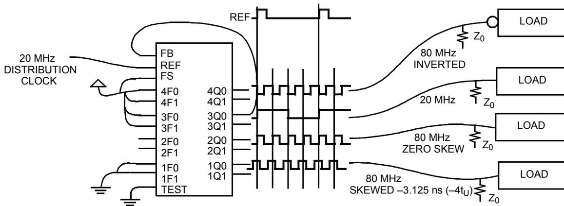
**Figure 10. Board-to-Board Clock Distribution**
