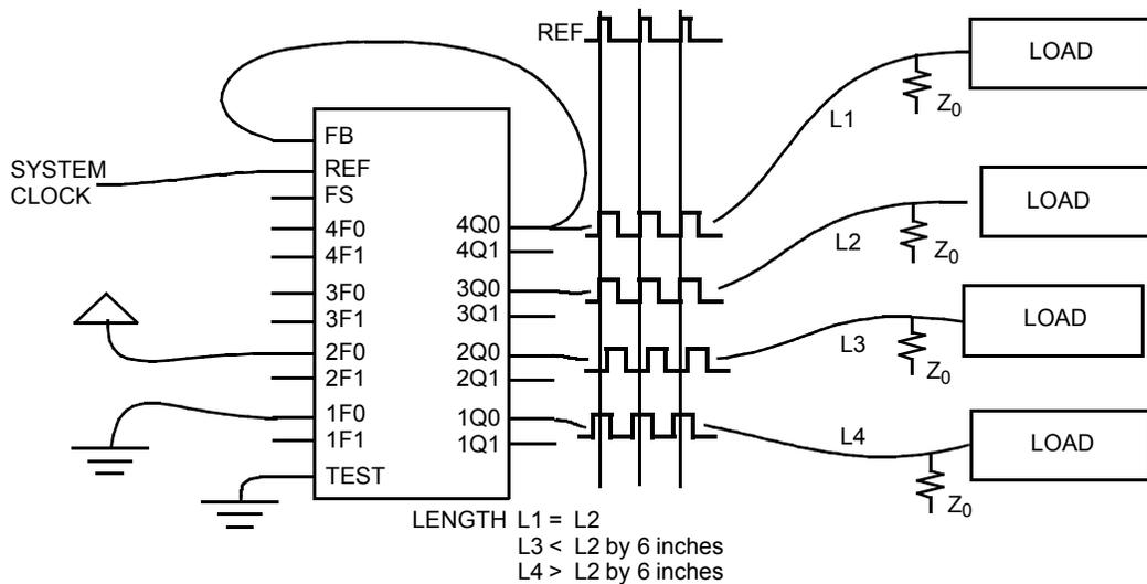
Figure 5 shows a configuration to equalize skew between metal traces of different lengths. In addition to low skew between outputs, the PSCB is programmed to stagger the timing of its
