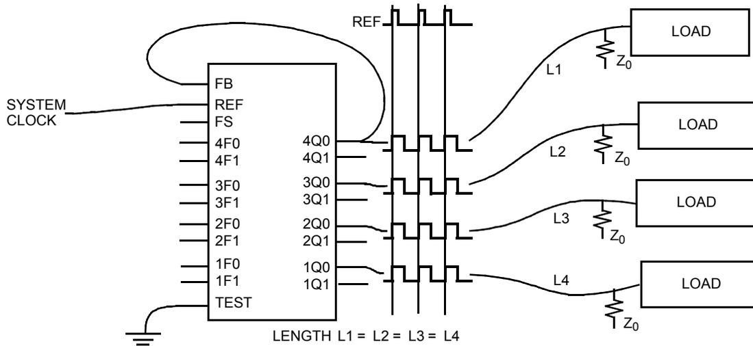
Figure 4 shows the PSCB configured as a zero skew clock buffer. In this mode the 7B991/992 is used as the basis for a low-skew clock distribution tree. When all of the function select inputs ( $\times F0$ ,  $\times F1$ ) are left open, the outputs are aligned and each drives a terminated transmission line to an independent load.
