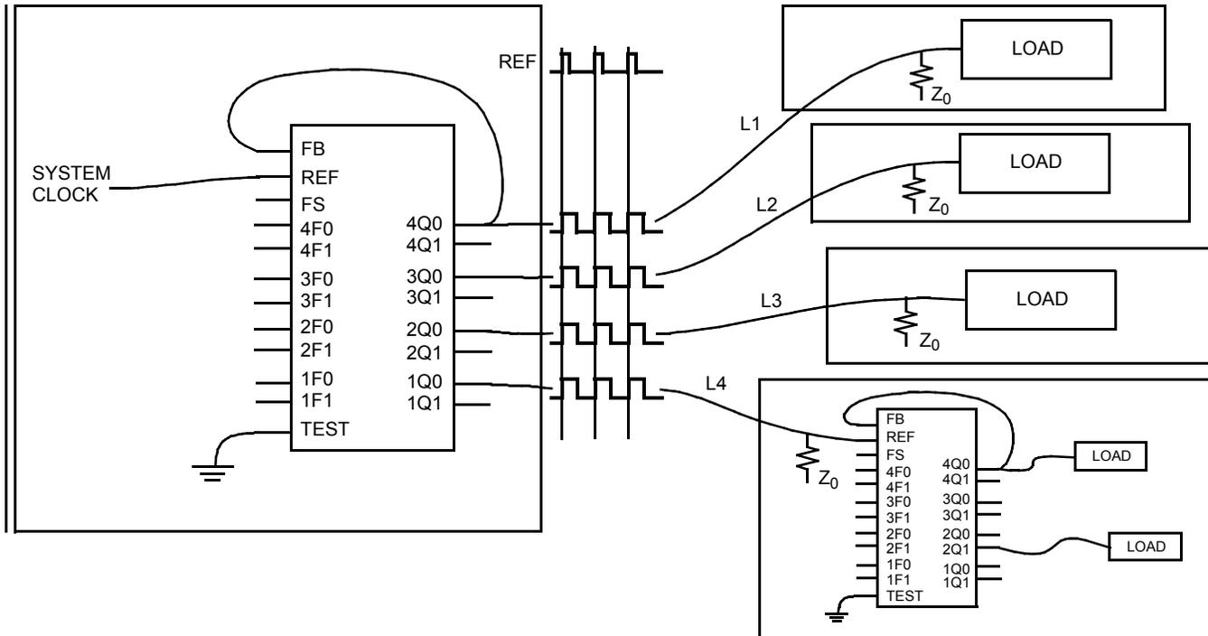
Figure 10 shows the CY7B991 and 992 connected in series to construct a zero skew clock distribution tree between boards. Delays of the downstream clock buffers are programmed to compensate for the wire length (that is, select negative skew equal to the wire delay) necessary to connect them to the master
