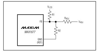
Figure 9. Adjusting LCD Output Voltage
