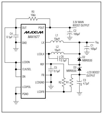
Figure 3. LCD Converter in Negative Mode
