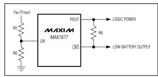
Figure 6. Setting the Low-Battery Trip Threshold
