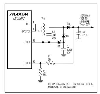
Figure 10. Higher LCD Output Voltage
