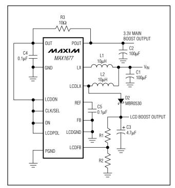
Figure 2. LCD Converter in Positive Mode
