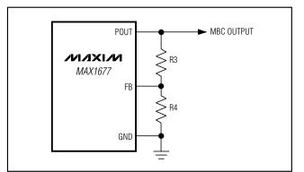
Figure 8. Setting the MBC Output Voltage Externally
