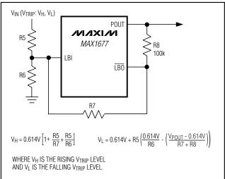
Figure 7. Adding External Hysteresis to the LBI Comparator
