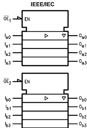
74F2244 Octal Buffer/Line Driver with 25Ω Series Resistors in Outputs
