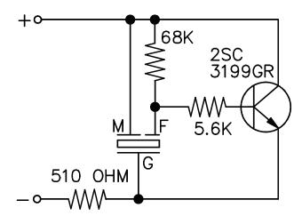
1. The current consumption and the sound pressure level are measured by using the recommended driving circuit shown above. Notes:
