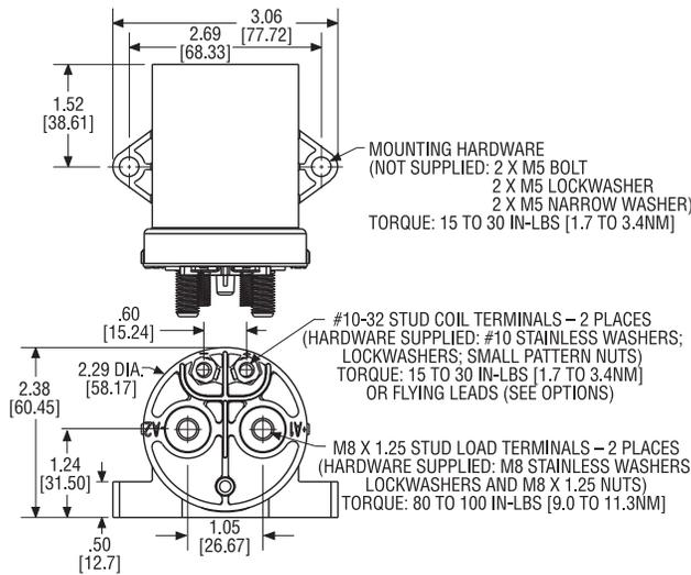
**Note:** When stud terminals are specified for coil connections, the electrical connection is made at the tab located at the base of the stud.
