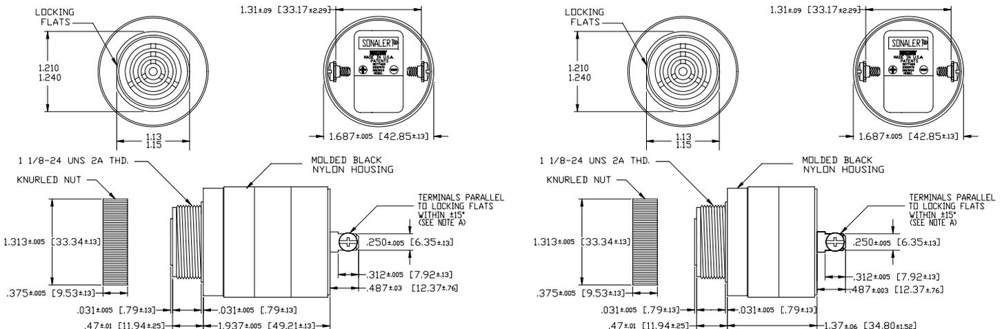
NOTE A: TERMINALS--032 BRASS TIN PLATED, TAPPED FOR #6-32 SCREW. TWO #6-32 NICKEL PLATED BRASS SCREWS INCLUDED. WILL ACCEPT 1/4" QUICK CONNECT.
