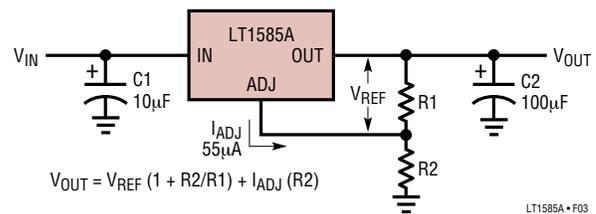
$$V_{OUT} = V_{REF} (1 + R2/R1) + I_{ADJ} (R2)$$
