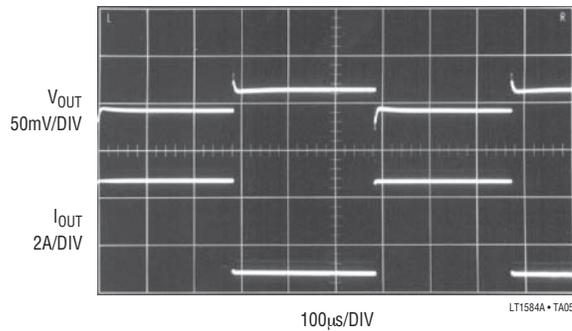
\* TRANSIENT RESPONSE MEASURED WITH AN INTEL POWER VALIDATOR.  $V_{OUT}$  IS MEASURED AT THE POWER VALIDATOR
