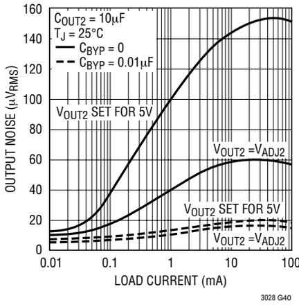
Output 1 RMS Output Noise vs Load Current (10Hz to 100kHz)
