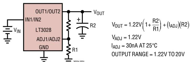
Figure 1. Adjustable Operation
