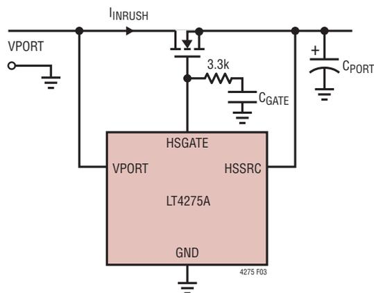
**Figure 3. Programming I<sub>INRUSH</sub>**
