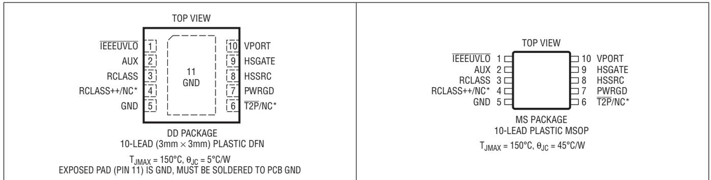
\* RCLASS++ is not connected in the LT4275B/C versions. T2P is not connected in the LT4275C version.
