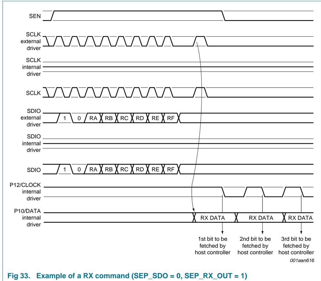
Fig 33. Example of a RX command (SEP\_SDO = 0, SEP\_RX\_OUT = 1)
