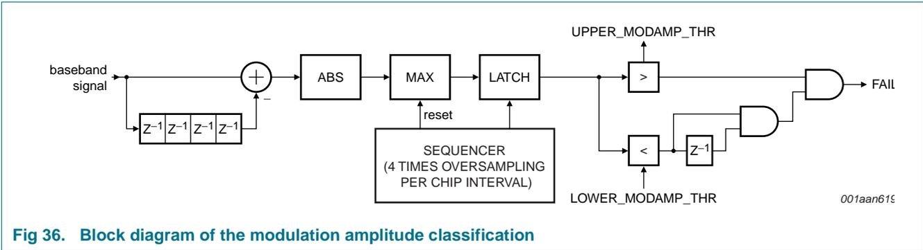
Fig 36. Block diagram of the modulation amplitude classification
