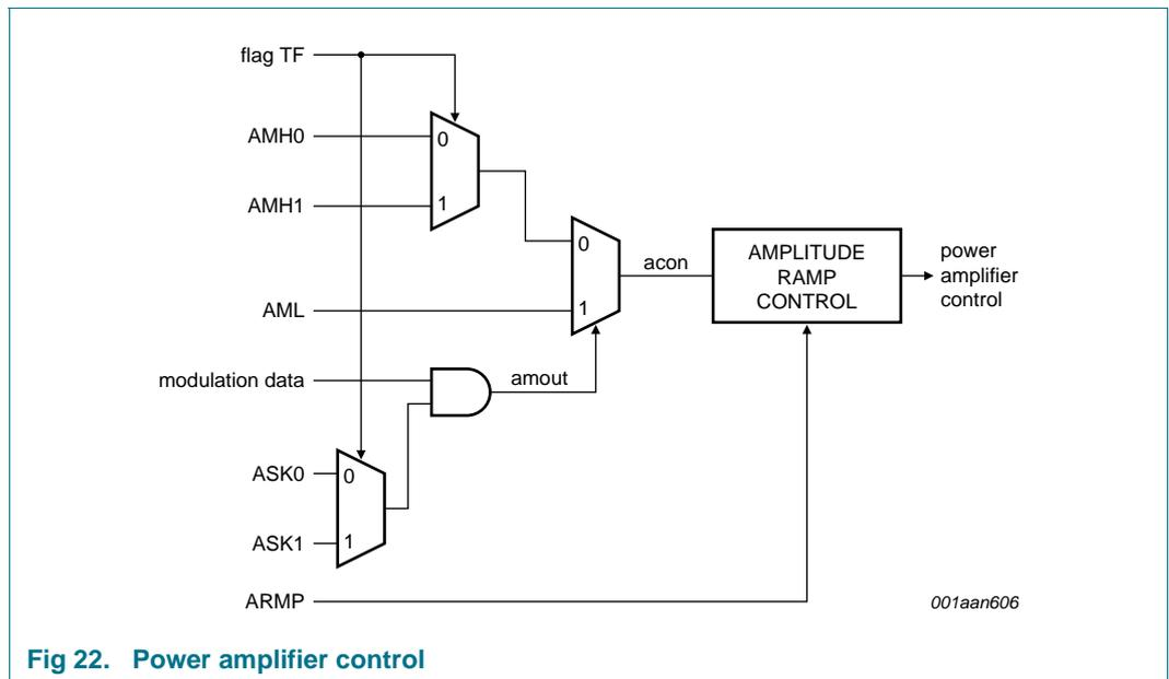
Fig 22. Power amplifier control
