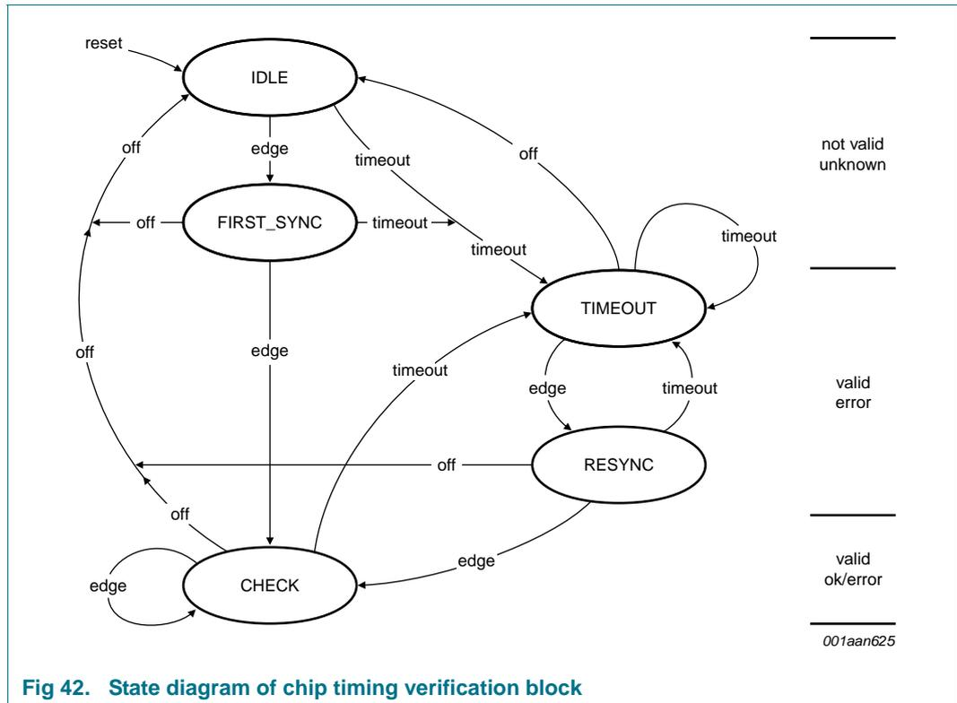
Fig 42. State diagram of chip timing verification block
