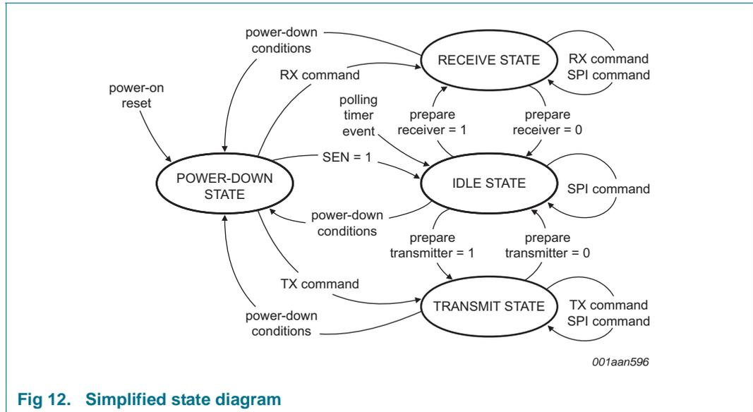
Fig 12. Simplified state diagram
