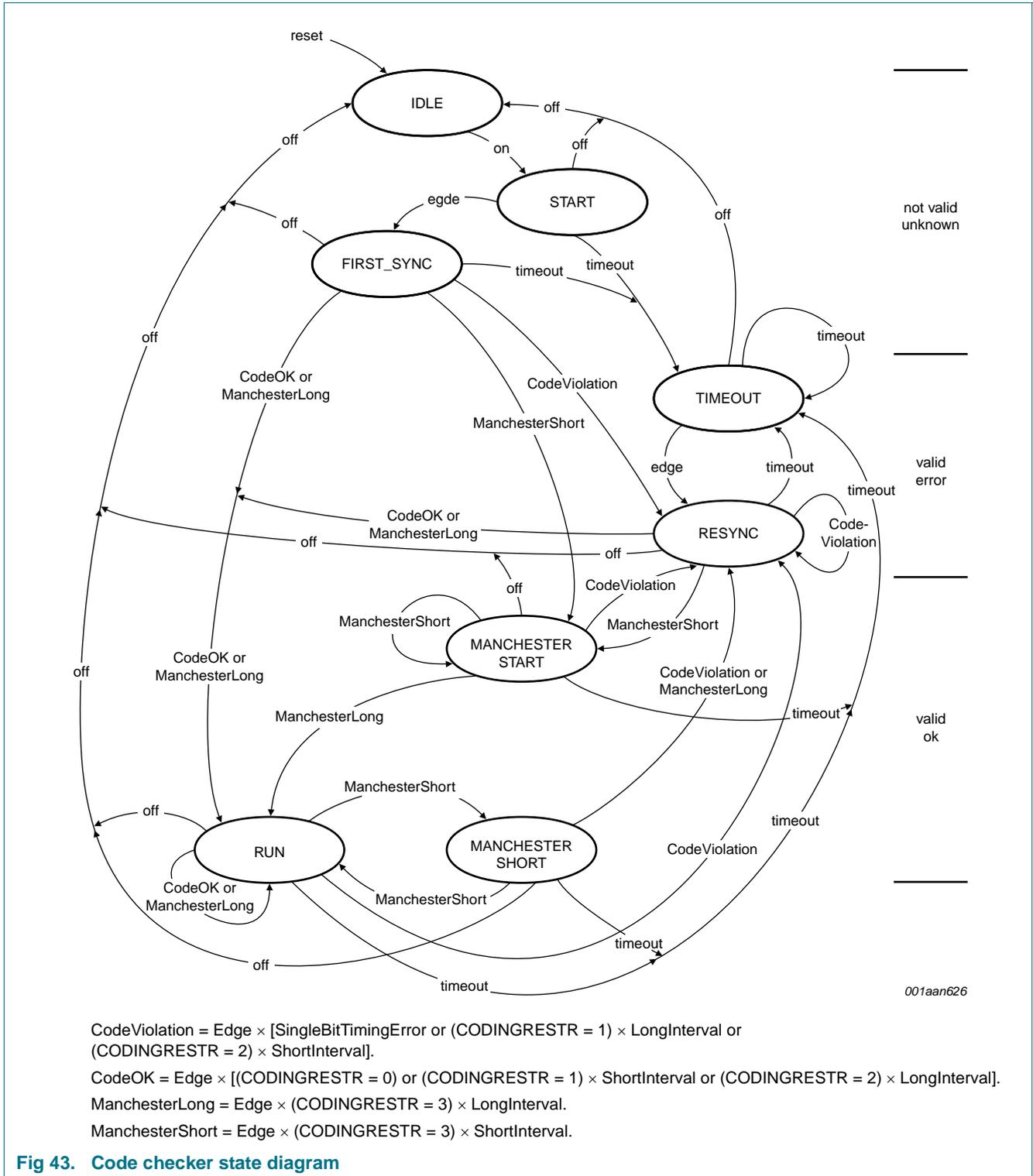
The timeout is derived from the chip timing verification block, i.e. a timeout is generated if a bit exceeds a length of  $3.5 \times$  chip width.
