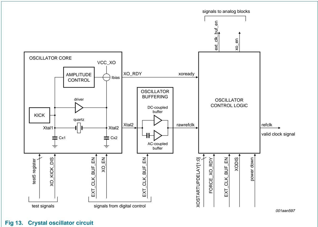
Fig 13. Crystal oscillator circuit
