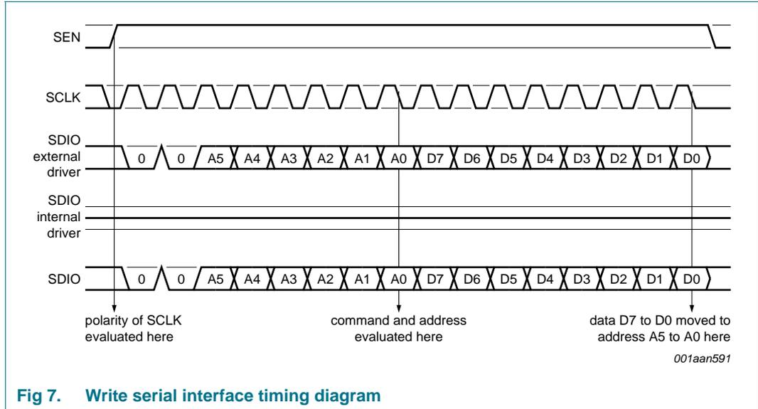
Fig 7. Write serial interface timing diagram
