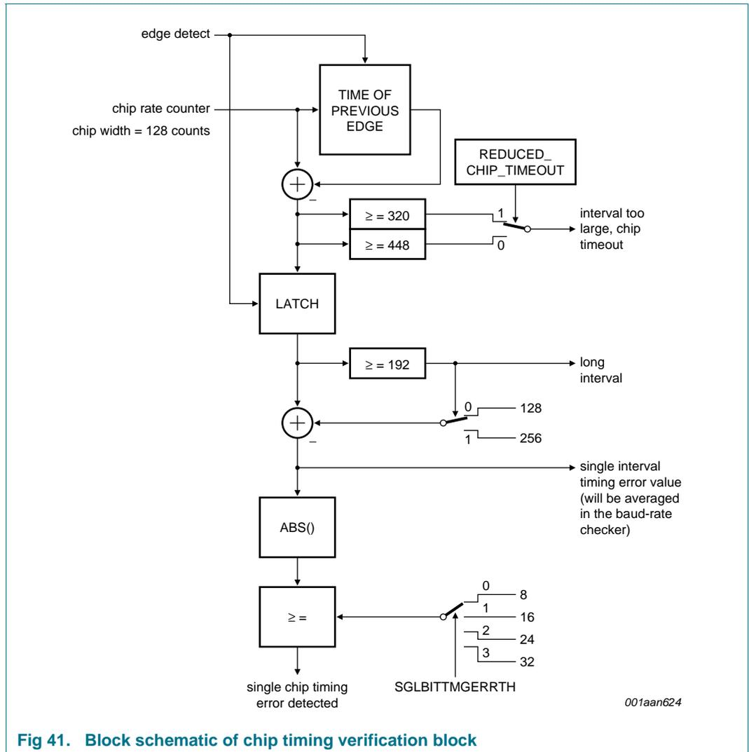
Fig 41. Block schematic of chip timing verification block
