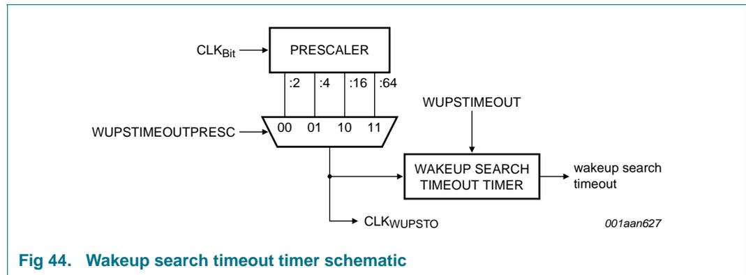
Fig 44. Wakeup search timeout timer schematic
