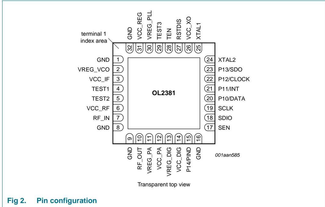
Fig 2. Pin configuration
