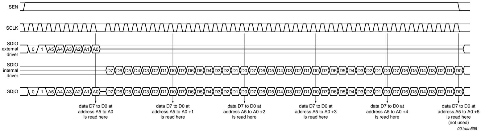
Fig 11. Read serial interface auto-increment timing diagram (SEP\_SDO = 0)
