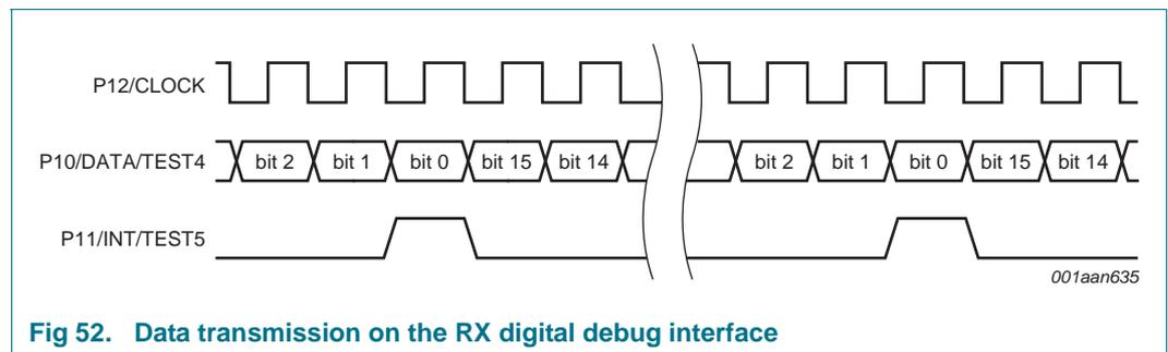
Fig 52. Data transmission on the RX digital debug interface
