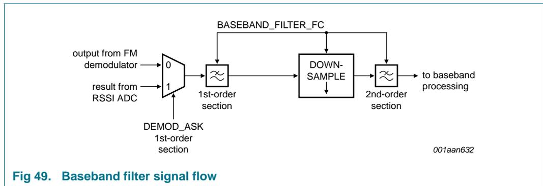
**Fig 49. Baseband filter signal flow**
