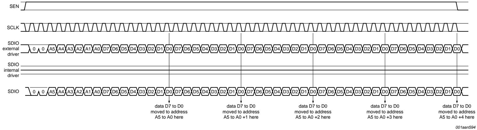
Fig 10. Write serial interface auto-increment timing diagram
