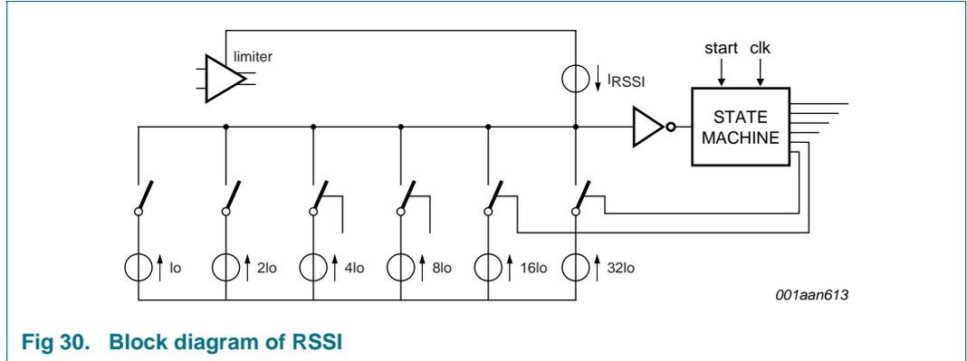
Fig 30. Block diagram of RSSI
