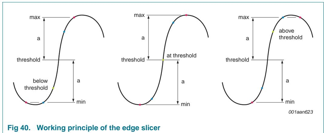
Fig 40. Working principle of the edge slicer
