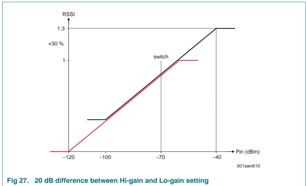
Fig 27. 20 dB difference between Hi-gain and Lo-gain setting
