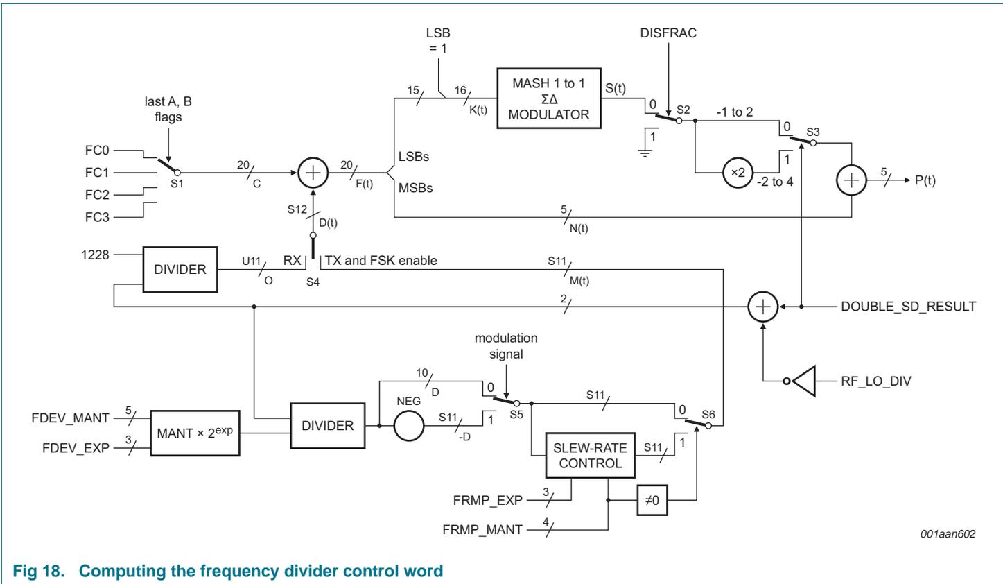
Fig 18. Computing the frequency divider control word
