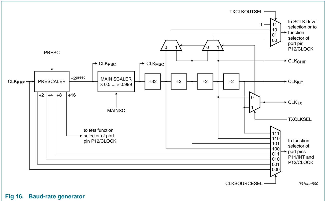
Fig 16. Baud-rate generator
