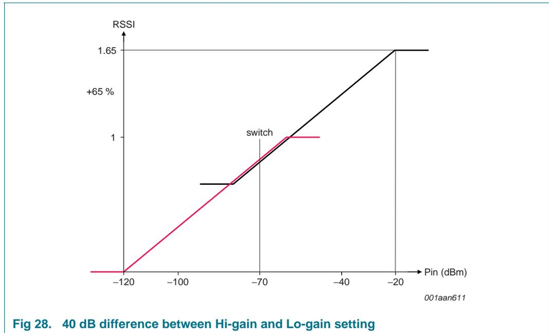
Fig 28. 40 dB difference between Hi-gain and Lo-gain setting
