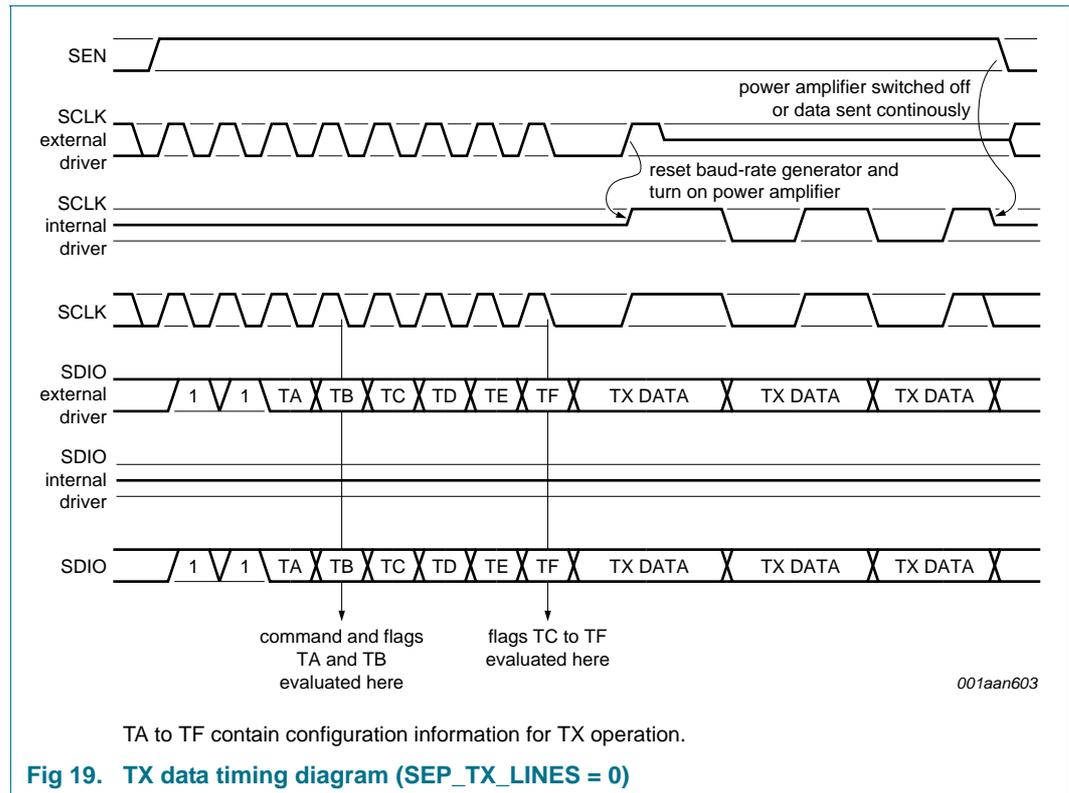
**Fig 19. TX data timing diagram (SEP\_TX\_LINES = 0)**
