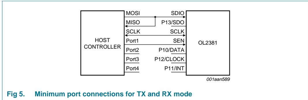
Fig 5. Minimum port connections for TX and RX mode
