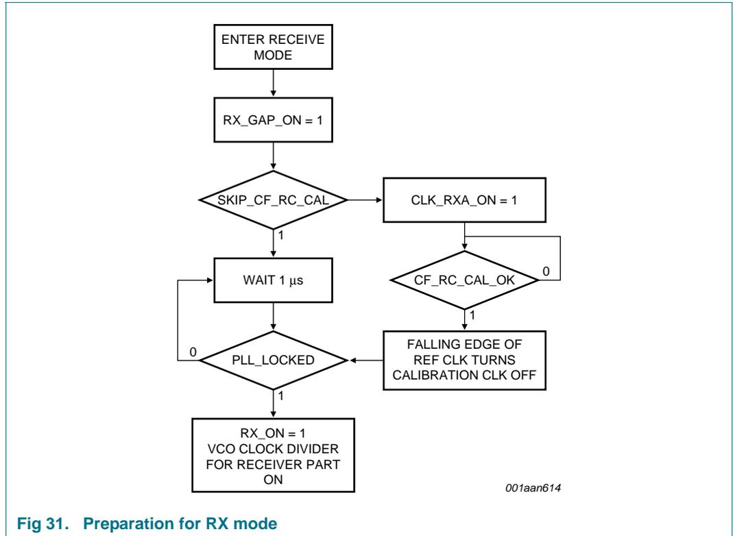
Fig 31. Preparation for RX mode
