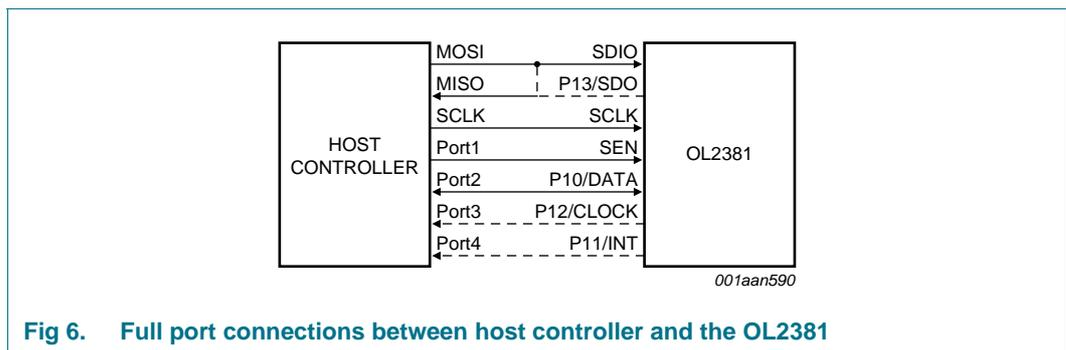
Fig 6. Full port connections between host controller and the OL2381
