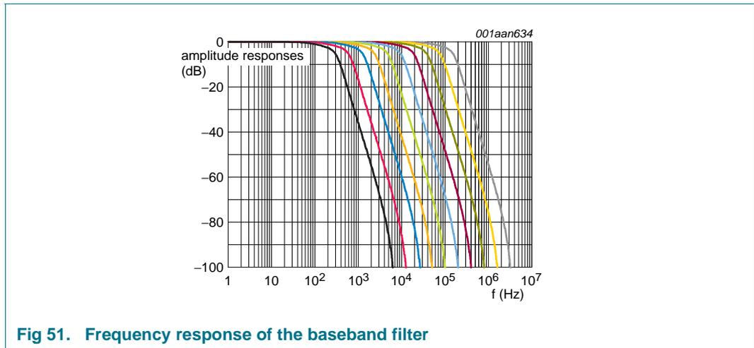
Fig 51. Frequency response of the baseband filter
