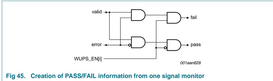
**Fig 45. Creation of PASS/FAIL information from one signal monitor**
