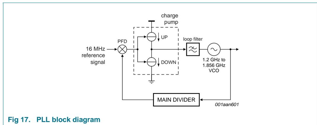
Fig 17. PLL block diagram
