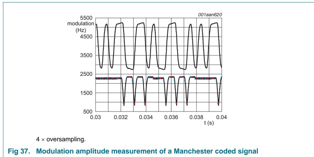
Fig 37. Modulation amplitude measurement of a Manchester coded signal
