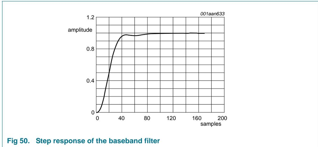
Fig 50. Step response of the baseband filter
