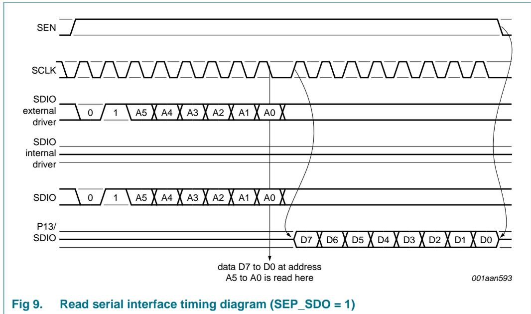
Fig 9. Read serial interface timing diagram (SEP\_SDO = 1)
