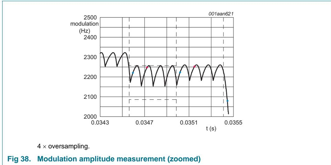
**Fig 38. Modulation amplitude measurement (zoomed)**
