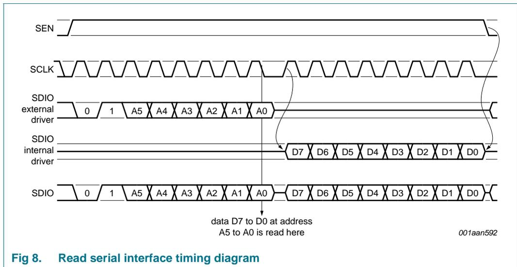
Fig 8. Read serial interface timing diagram
