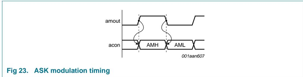
Fig 23. ASK modulation timing
