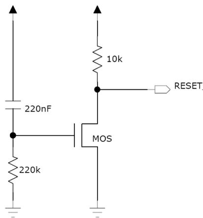
**Figure 23: Example of a simple power on reset circuit.**
