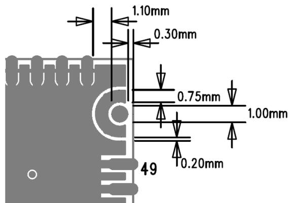
Figure 5: Dimensions for the RF pin (top view)
