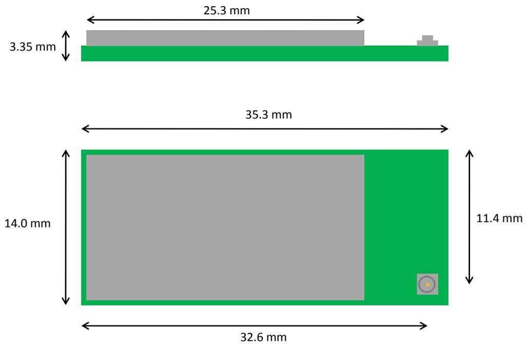
**Figure 6: Dimensions of WT41-E**
