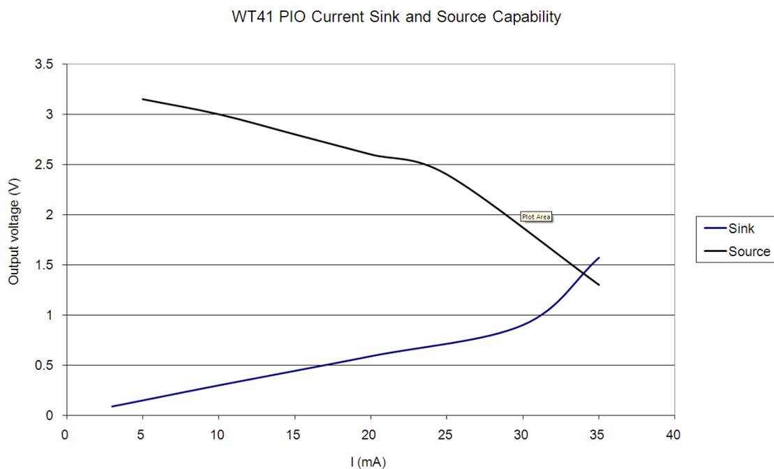
Figure 2: WT41-E PIO Current Drive Capability
