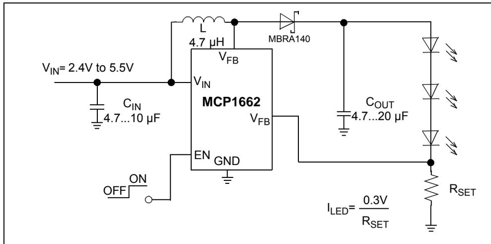
**FIGURE 1-1:** Typical MCP1662 LED Driver Boost Converter Application.
