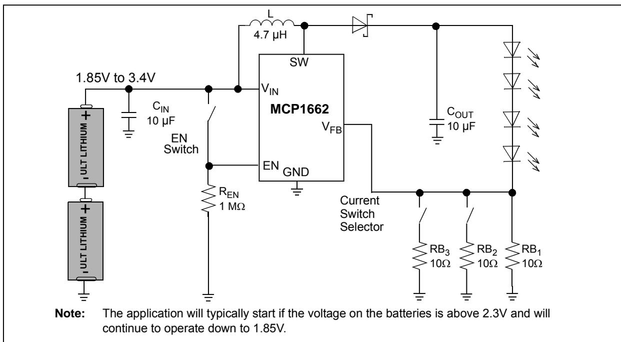
**FIGURE 2-1:** MCP1662 Boost 30, 60, 90 mA Constant Current Application.
