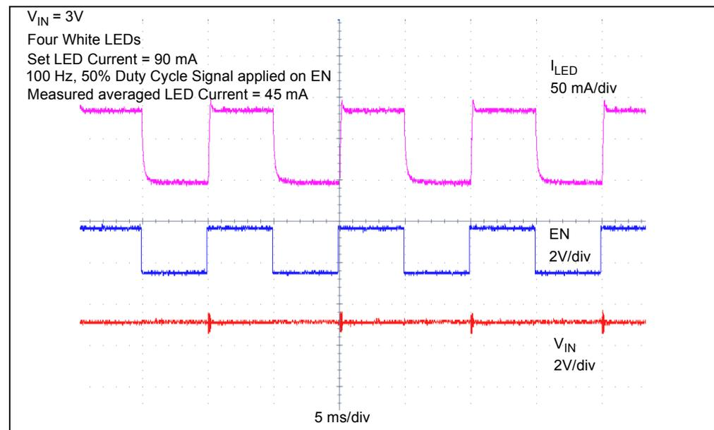
**FIGURE 2-3:** PWM Dimming with MCP1662.
