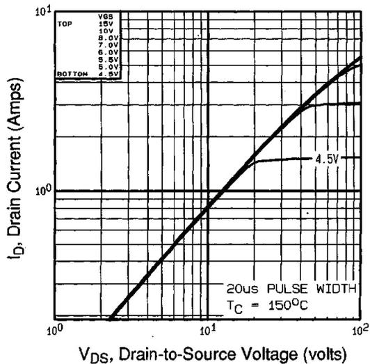
**Fig. 2 - Typical Output Characteristics,  $T_C = 150\text{ }^\circ\text{C}$**
