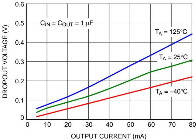
Figure 13. NCP716x50xxx Dropout Voltage vs. Output Current
