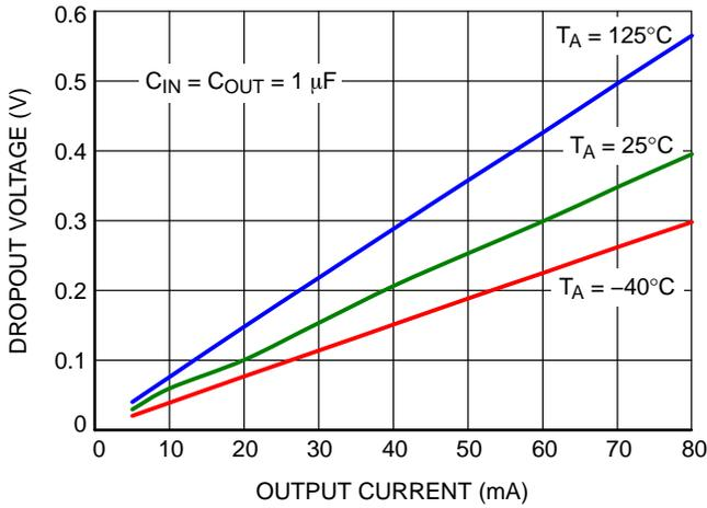
Figure 11. NCP716x25xxx Dropout Voltage vs. Output Current
