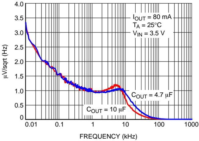
Figure 27. NCP716x25xxx Output Spectral Noise Density vs. Frequency
