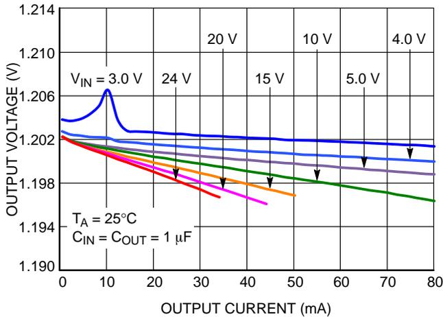
Figure 7. NCP716x12xxx Output Voltage vs. Output Current
