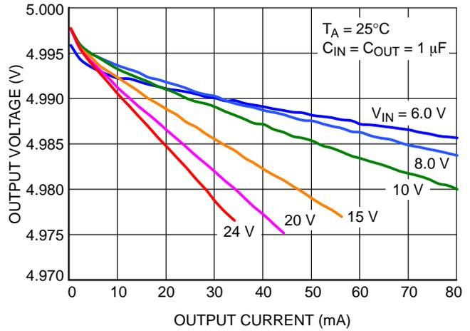
Figure 10. NCP716x50xxx Output Voltage vs. Output Current
