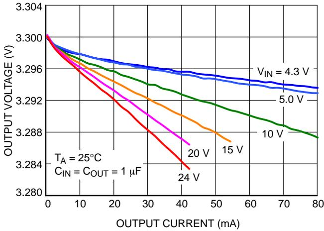
Figure 9. NCP7163V3 Output Voltage vs. Output Current
