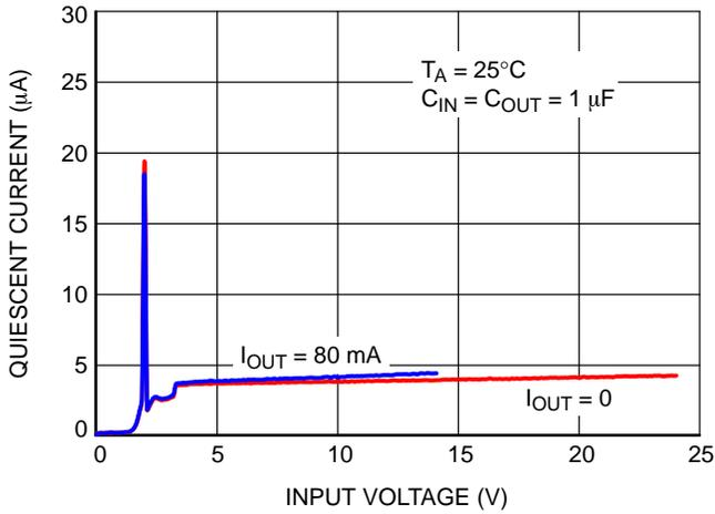
Figure 17. NCP716x33xxx Ground Current vs. Input Voltage
