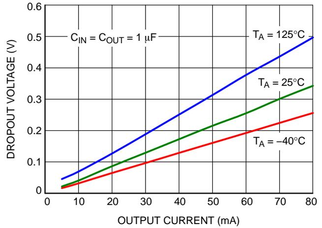
Figure 12. NCP716x33xxx Dropout Voltage vs. Output Current
