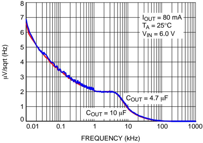
Figure 29. NCP716x50xxx Output Spectral Noise Density vs. Frequency
