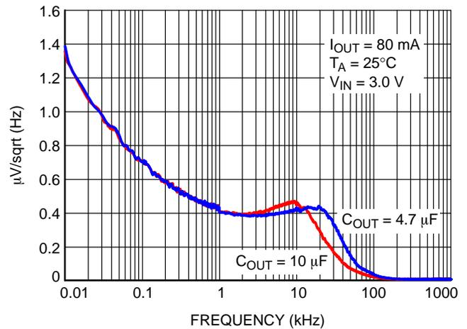
**Figure 26. NCP716x12xxx Output Spectral Noise Density vs. Frequency**
