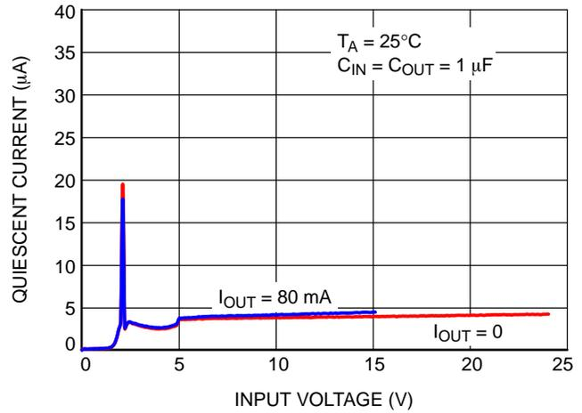
Figure 16. NCP716x50xxx Ground Current vs. Input Voltage
