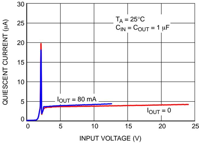
Figure 15. NCP716x25xxx Ground Current vs. Input Voltage
