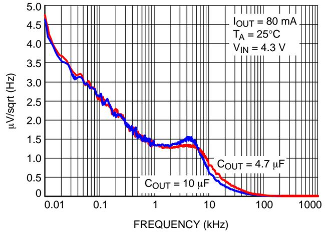
Figure 28. NCP716x33xxx Output Spectral Noise Density vs. Frequency
