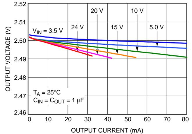
Figure 8. NCP716x25xxx Output Voltage vs. Output Current
