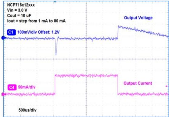
Figure 30. Load Transient Response
