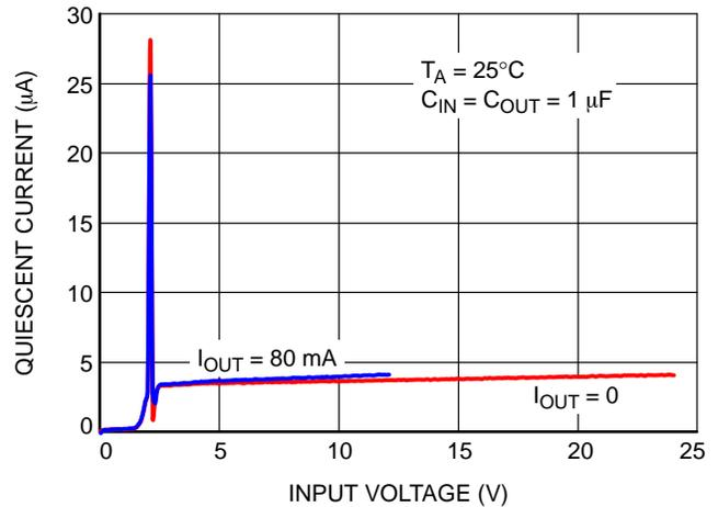
Figure 14. NCP716x12xxx Ground Current vs. Input Voltage
