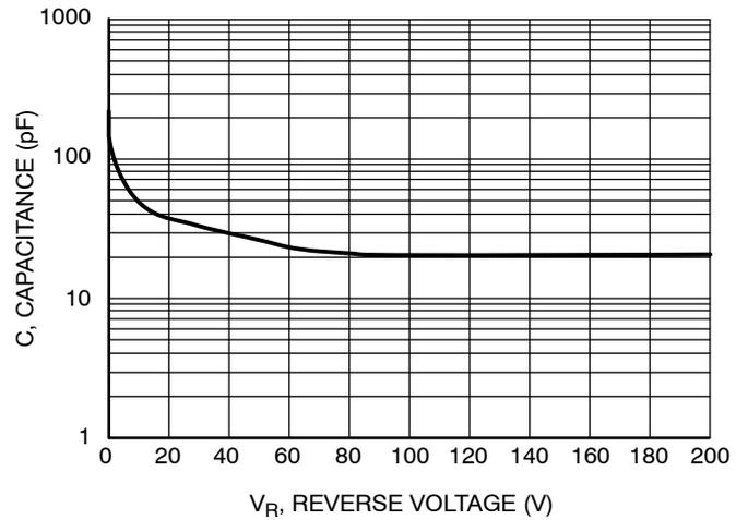
Figure 2. Typical Capacitance
