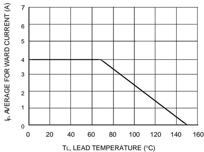
**Figure 5. Derating Curve**
