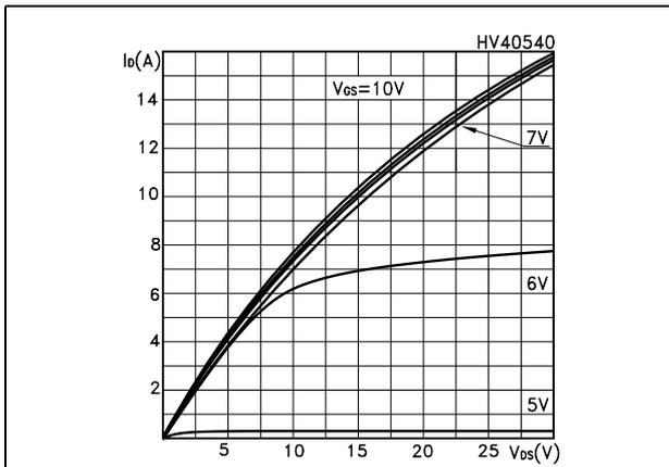
Figure 5. Transfer characteristics
