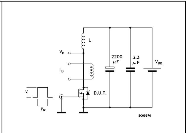
Figure 18. Unclamped inductive waveform
