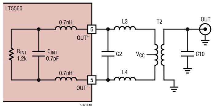
Figure 10. Output Port Small-Signal Model with External Matching
