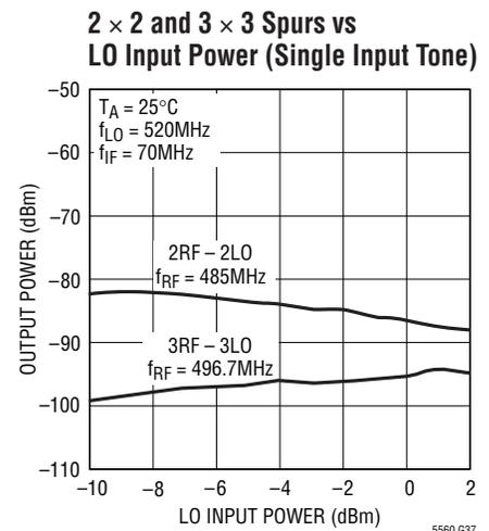
**TYPICAL AC PERFORMANCE CHARACTERISTICS** 1900MHz Downconverting Mixer Application:
