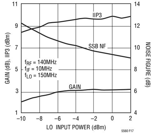
**Figure 17. LT5560 Performance in 140MHz Downconverting Mixer Application**
