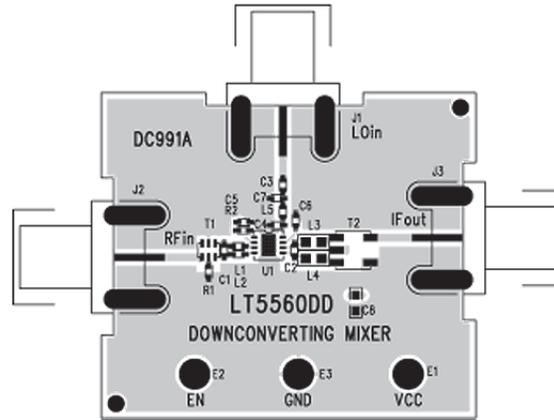
Figure 24. Downconverting Mixer Evaluation Board (DC991A)—See Table 1
