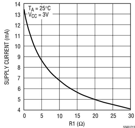
Figure 13. Typical Supply Current vs R1 Value
