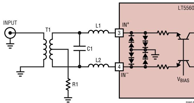
**Figure 4. Input Port with Lowpass External Matching Topology**
