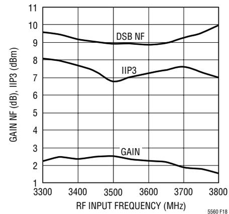
**Figure 18. LT5560 Performance as a 3600MHz Downconverting Mixer**
