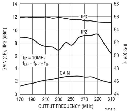
**Figure 16. LT5560 Performance in 240MHz Upconverting Mixer Application**
