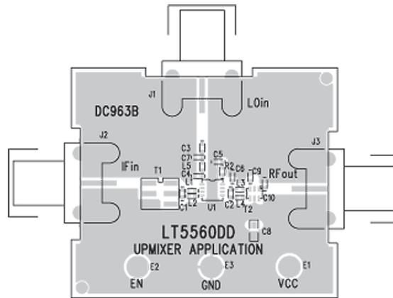
Figure 23. Upconverting Mixer Evaluation Board (DC963B)—See Table 1
