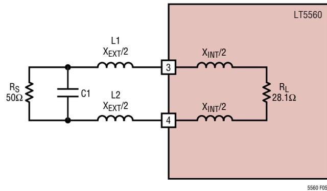
Figure 5. Small Signal Circuit for the Input Port
