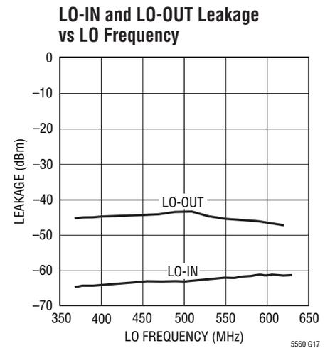
**1900MHz Upconverting Mixer Application:  $V_{CC} = 3V$ ,  $I_{CC} = 10mA$ ,  $EN = 3V$ ,  $T_A = 25^\circ C$ ,  $f_{IN} = 140MHz$ ,  $P_{IN} = -20dBm$  (-20dBm/tone for 2-tone IIP3 tests,  $\Delta f = 1MHz$ ),  $f_{LO} = 1760MHz$ ,  $P_{LO} = -2dBm$ , output measured at 1900MHz, unless otherwise noted. (Test circuit shown in Figure 1)**
