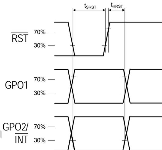
**Figure 1. Reset Timing Parameters for Busmode Select**
