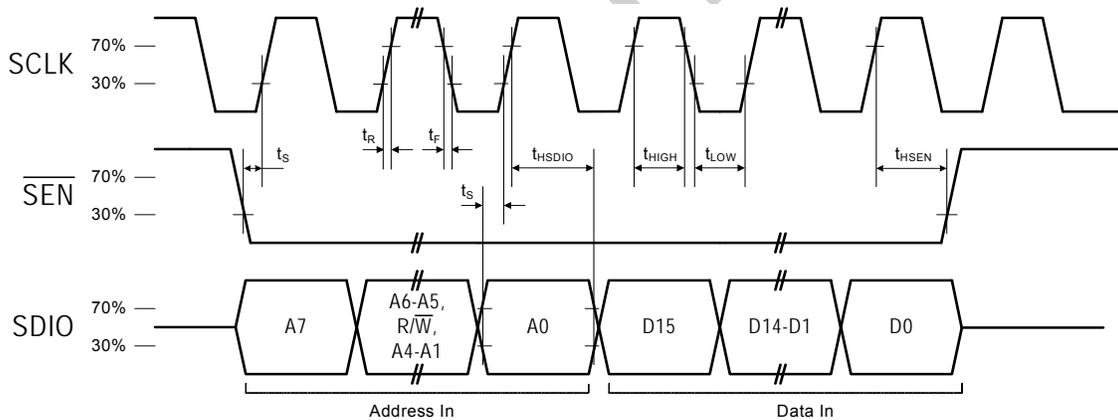
**Figure 4. 3-Wire Control Interface Write Timing Parameters**
