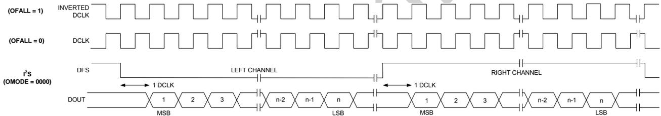
Figure 10. I<sup>2</sup>S Digital Audio Format
