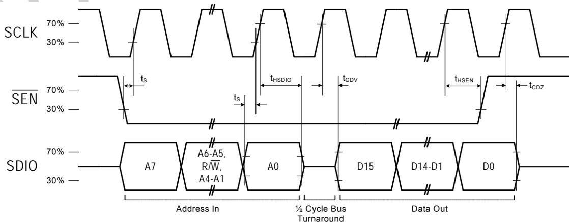
**Figure 5. 3-Wire Control Interface Read Timing Parameters**
