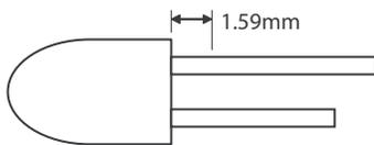
Soldering the LED using soldering iron tip closer than 1.59mm might damage the LED.
