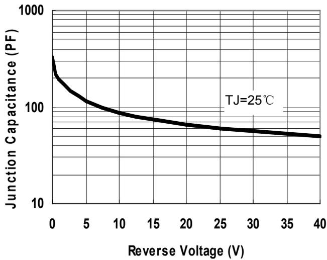
**Fig.1-Typical Junction Capacitance**
