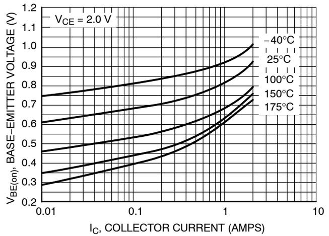
Figure 5. Base-Emitter Voltage
