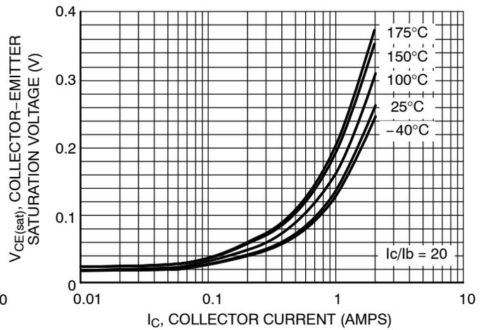
Figure 3. Collector-Emitter Saturation Voltage
