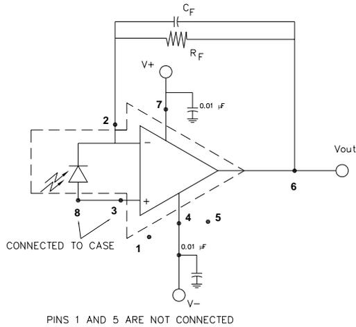
**Note:** Components shown outside the dashed area are external to the device, and must be supplied by the user.
