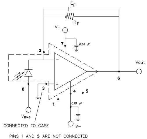
**Note:** Components shown outside the dashed area are external to the device, and must be supplied by the user.
