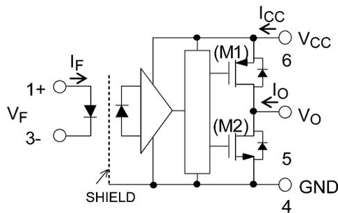
Note: A 1- $\mu$ F bypass capacitor must be connected between pin 6 and pin 4.
