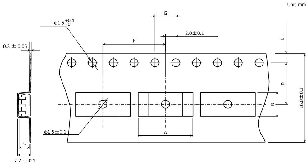
**Table Tape Dimensions (unit: mm, tolerance: ± 0.1)**
