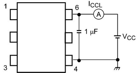
**Fig. 12.1.6 I<sub>CCL</sub> Test Circuit**
