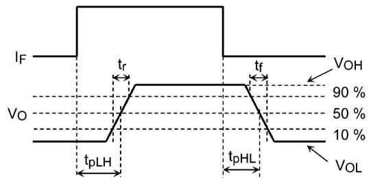
**Fig. 12.1.7 Switching Time Test Circuit and Waveform**
