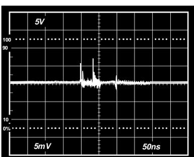
Figure 15. Crosstalk— $V_{OUT}$  @ 5 mV/Div
