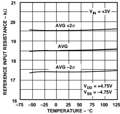
Figure 7. Input Resistance ( $V_{IN}$ ) vs. Temperature
