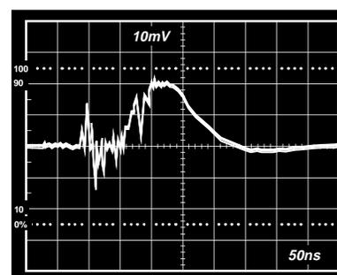
Figure 17. Digital Feedthrough— $V_{OUT}$  @ 10 mV/Div,
