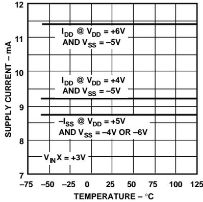
Figure 22. Supply Current vs. Voltage and Temperature
