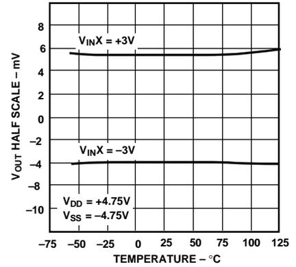
Figure 6.  $V_{OUT}$  Half Scale ( $80_H$ ) vs. Temperature
