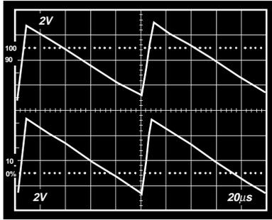
Figure 19. 10 kHz Sawtooth Waveform, Upper Trace  $V_{IN}$ , Lower Trace  $V_{OUT}$
