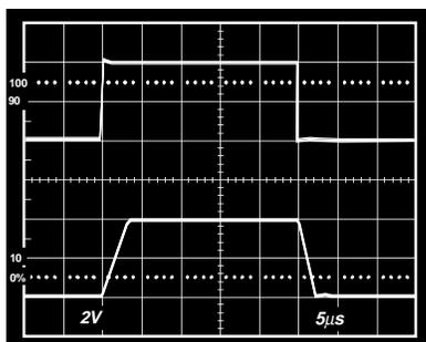
Figure 13. Pulse Response—Upper Trace  $V_{IN}$  @ 2 V/Div
