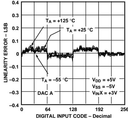
Figure 5. Linearity Error vs. Digital Code vs. Temperature
