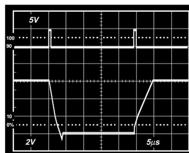
Figure 16. Settling Time—Upper Trace LD @ 5 V/Div,
