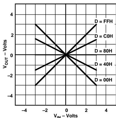
$$V_{OUT} = V_{IN} (D/128 - 1), \text{ WHERE } D = 0 \text{ TO } 255$$
