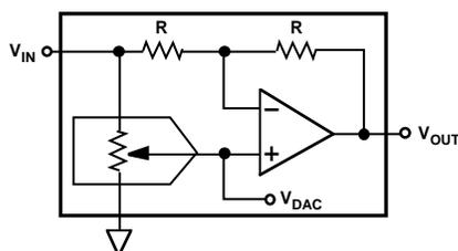
$$\begin{aligned} V_{DAC} &= D/256 \times V_{IN} \\ V_{OUT} &= 2 \times V_{DAC} - V_{IN} \\ &= 2 (D/256) \times V_{IN} - V_{IN} \\ &= (D/128 - 1) \times V_{IN} \end{aligned}$$
