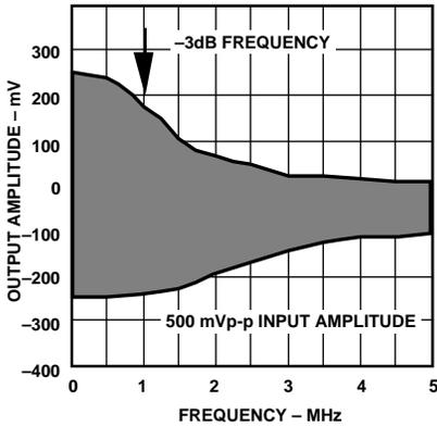
Figure 21. AC Sweep Frequency 500 mV p-p Amplitude Response
