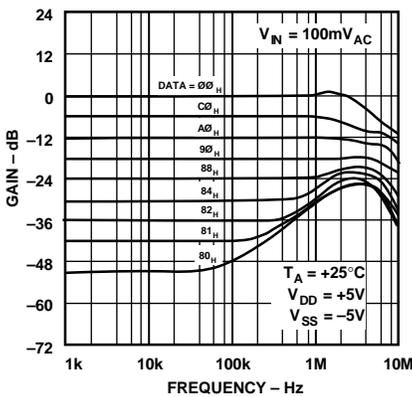
Figure 24. Gain ( $V_{OUT}/V_{IN}$ ) and Feedthrough vs. Frequency
