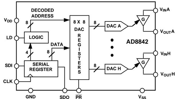
The AD8842 consumes only 95 mW from  $\pm 5$  V power supplies. For single 5 V supply applications consult the DAC-8841. The AD8842 is pin compatible with the 1 MHz multiplying bandwidth DAC8840. The AD8842 is available in 24-pin plastic DIP and surface mount SOL-24 packages.
