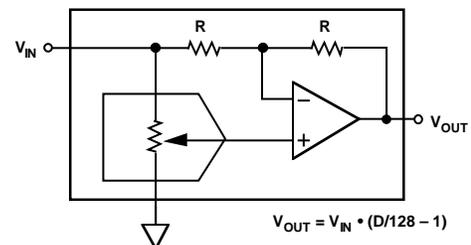
Figure 1. Functional Circuit of One 4-Quadrant Multiplying Channel
