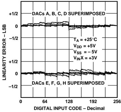
Figure 4. Linearity Error vs. Digital Code
