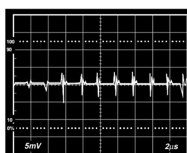
Figure 18. Clock Feedthrough— $V_{OUT}$  @ 5 mV/Div
