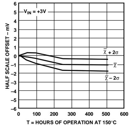
Figure 26. Output Voltage Drift Accelerated by Burn-In
