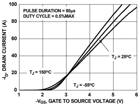
Figure 5. Transfer Characteristics
