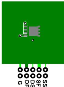
a.  $45^\circ\text{C}/\text{W}$  when mounted on a 1 in<sup>2</sup> pad of 2 oz copper.
