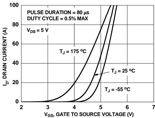
Figure 5. Transfer Characteristics
