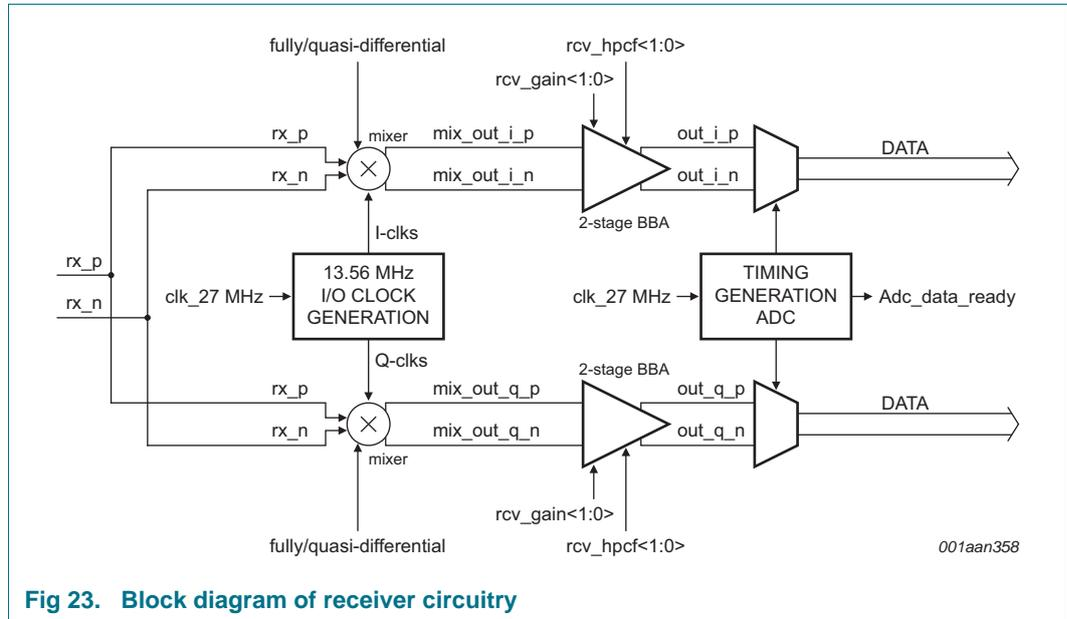
Fig 23. Block diagram of receiver circuitry
