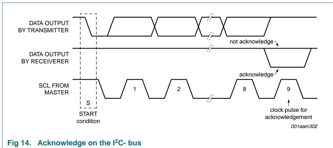
Fig 14. Acknowledge on the I<sup>2</sup>C- bus
