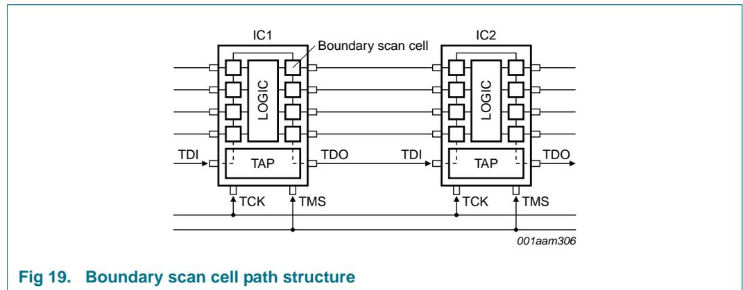
Fig 19. Boundary scan cell path structure
