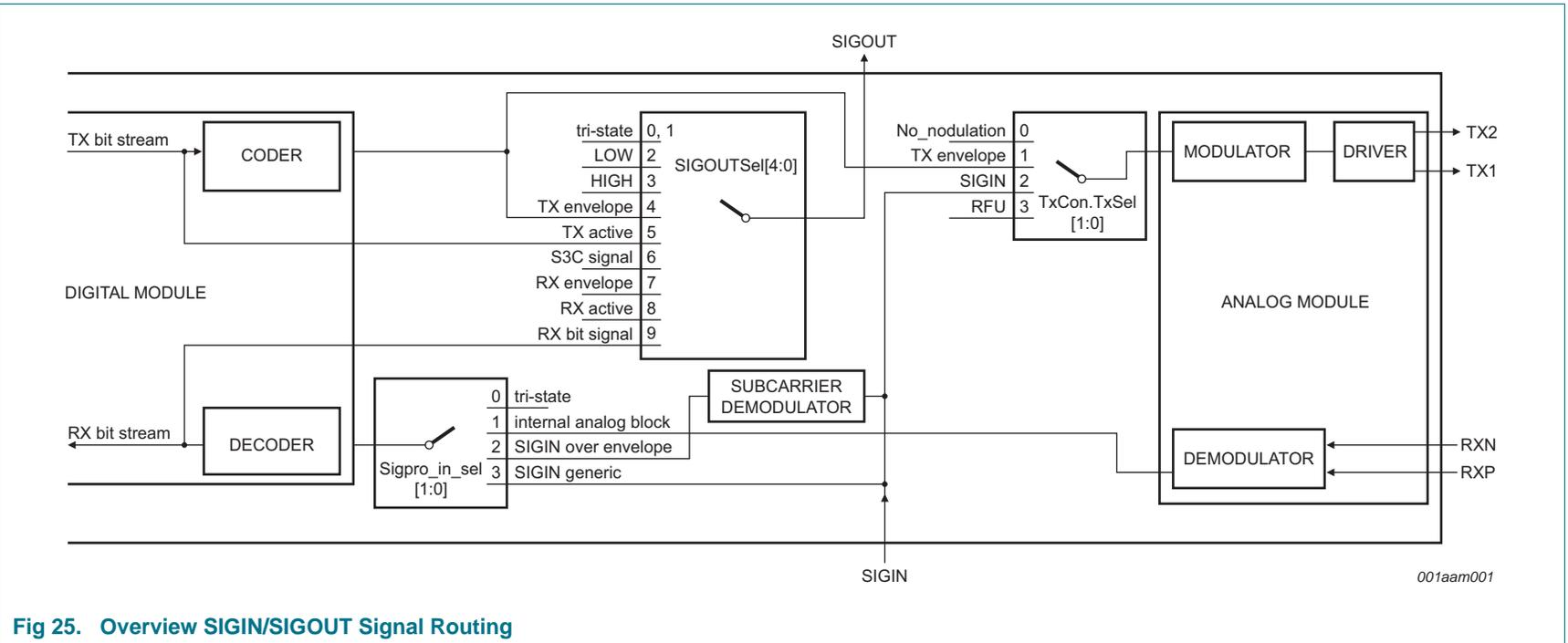
Fig 25. Overview SIGIN/SIGOUT Signal Routing
