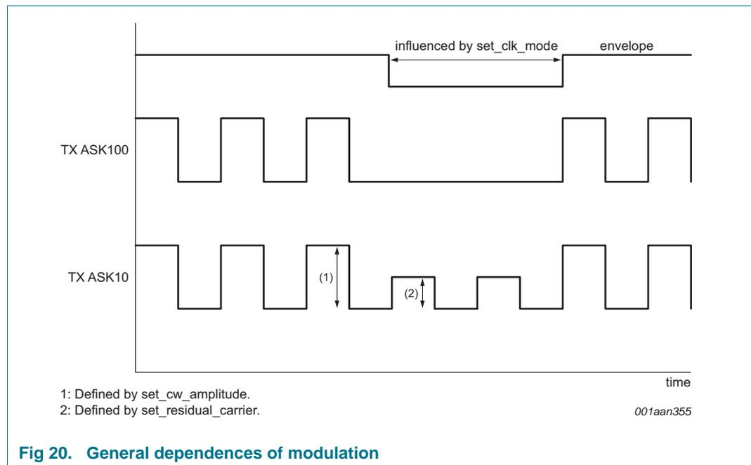
Fig 20. General dependences of modulation
