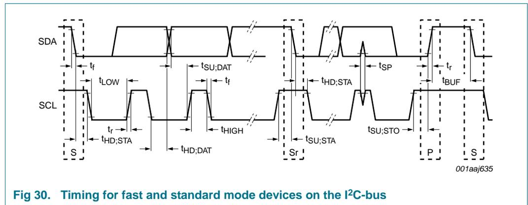
**Fig 30. Timing for fast and standard mode devices on the I<sup>2</sup>C-bus**
