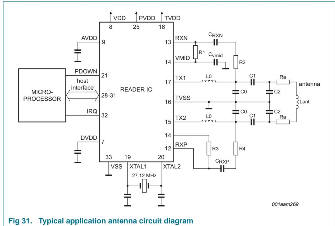
Fig 31. Typical application antenna circuit diagram
