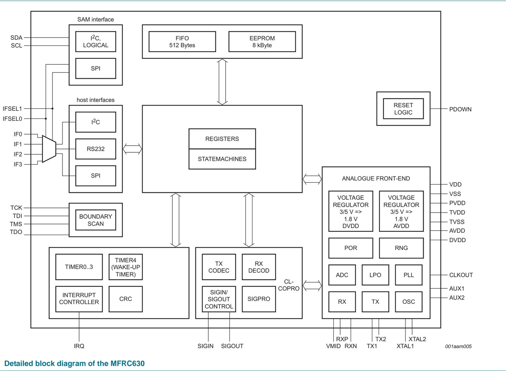
Fig 3. Detailed block diagram of the MFR630
