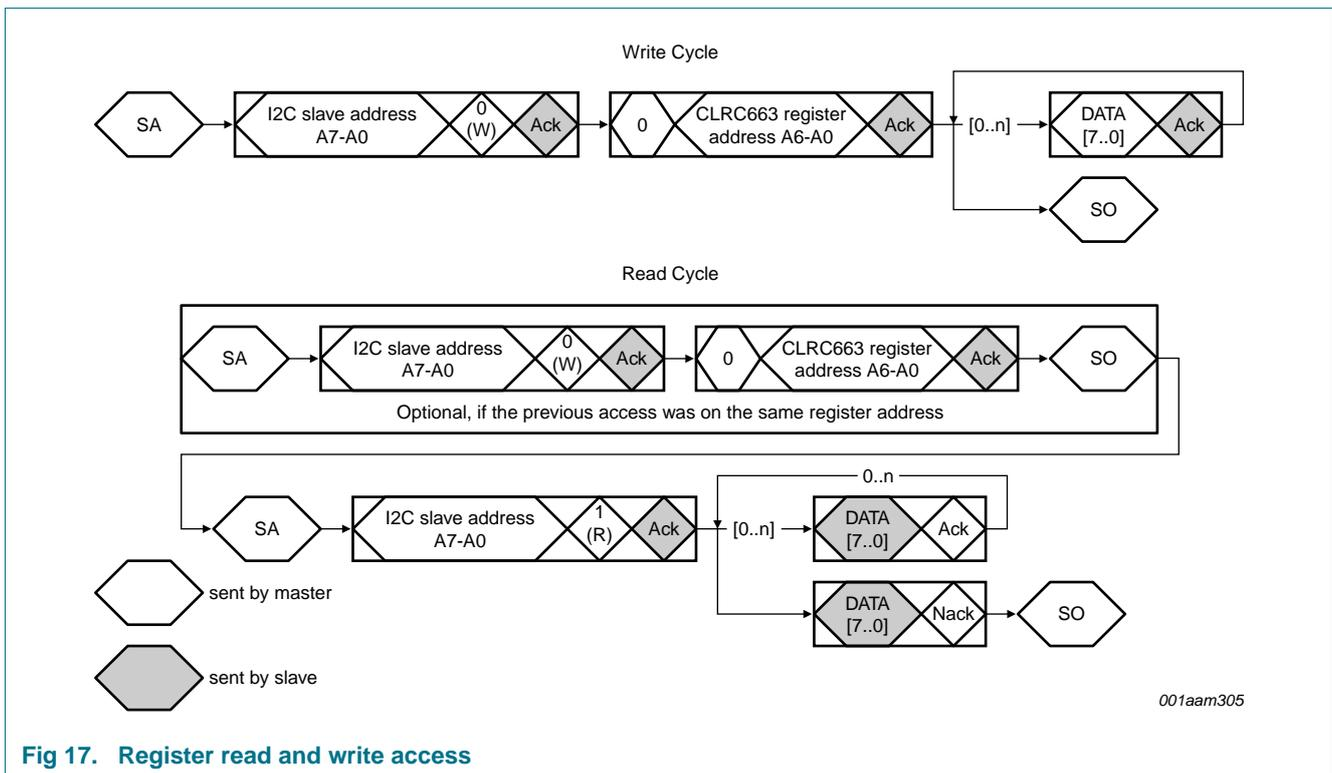
Fig 17. Register read and write access
