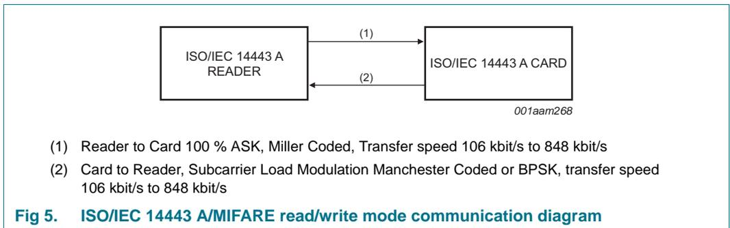
**Fig 5. ISO/IEC 14443 A/MIFARE read/write mode communication diagram**
