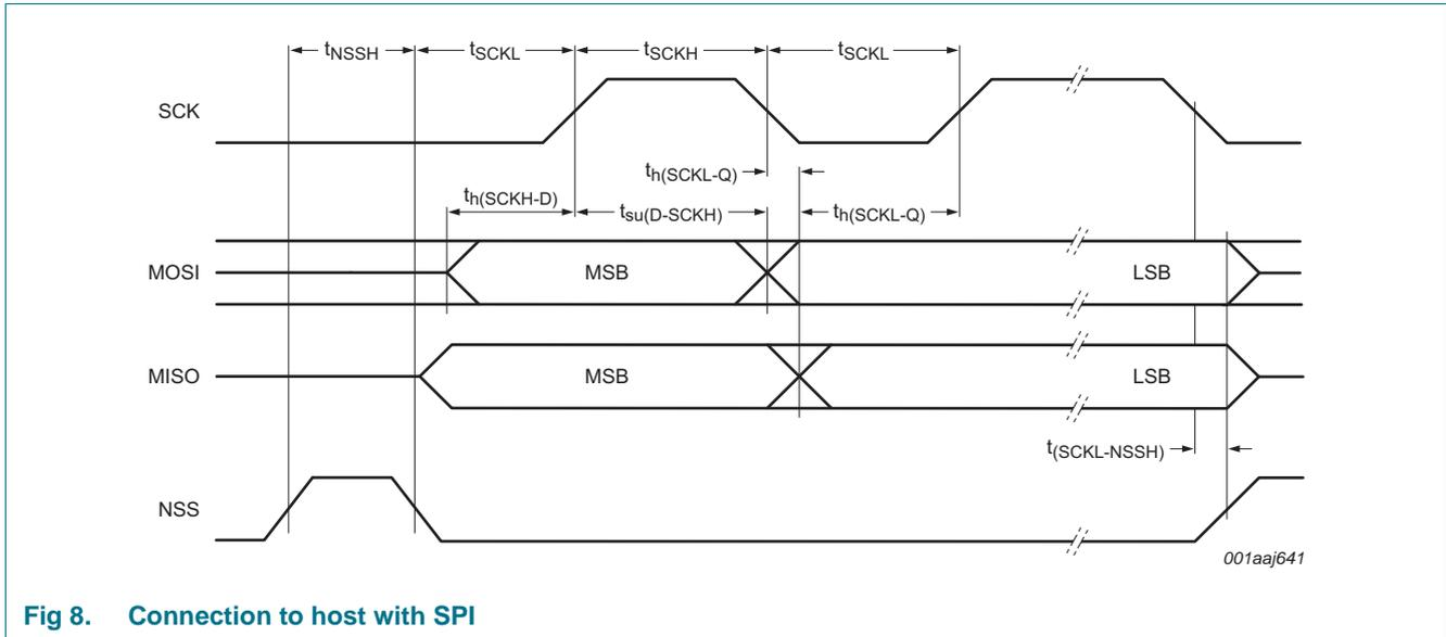
Fig 8. Connection to host with SPI
