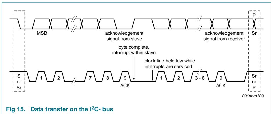
Fig 15. Data transfer on the I<sup>2</sup>C- bus
