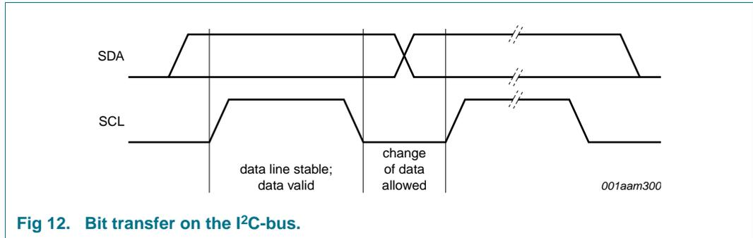
Fig 12. Bit transfer on the I<sup>2</sup>C-bus.
