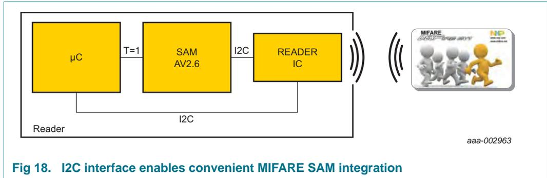
**Fig 18. I2C interface enables convenient MIFARE SAM integration**
