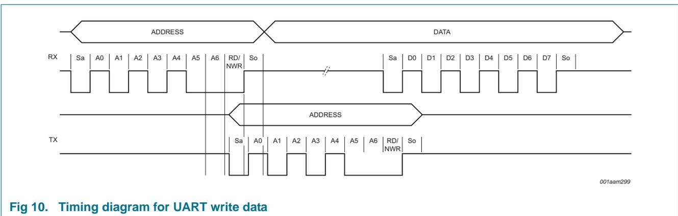
Fig 10. Timing diagram for UART write data
