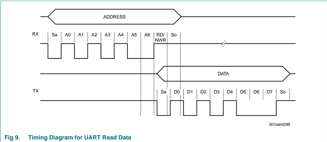
Fig 9. Timing Diagram for UART Read Data
