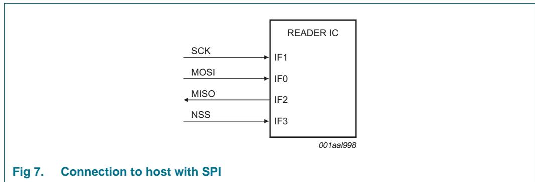
**Fig 7. Connection to host with SPI**
