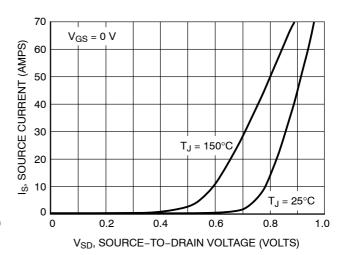
Figure 10. Diode Forward Voltage versus Current
