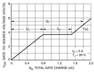
Figure 8. Gate-to-Source and Drain-to-Source Voltage versus Total Charge
