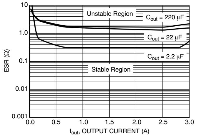
Figure 12. Output Capacitor ESR Stability vs. Output Current
