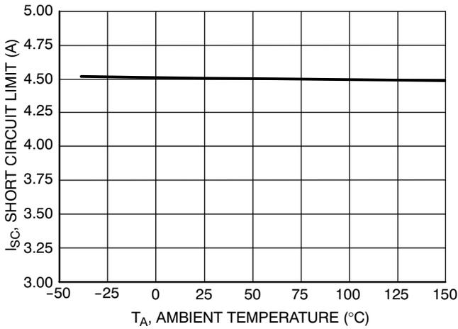
Figure 9. Short Circuit Current Limit vs. Ambient Temperature
