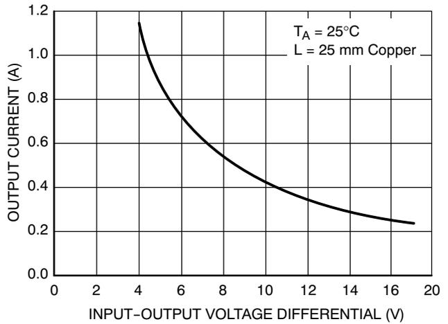
Figure 10. Output Current vs. Input-Output Voltage Differential
