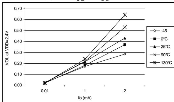
Figure 74. Typical  $V_{OL}$  at  $V_{DD}=2.7V$  (standard)
