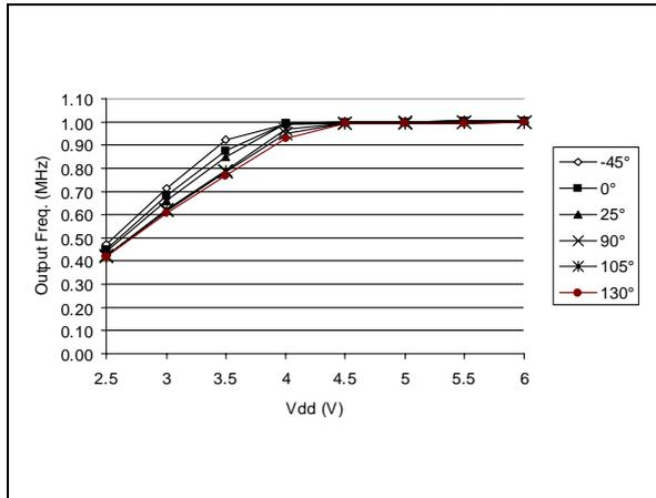
Figure 55. Typical RC oscillator Accuracy vs temperature @  $V_{DD}=5\text{V}$
