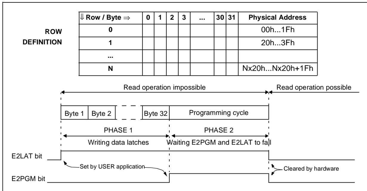
**Note:** If a programming cycle is interrupted (by software or a reset action), the integrity of the data in memory is not guaranteed.
