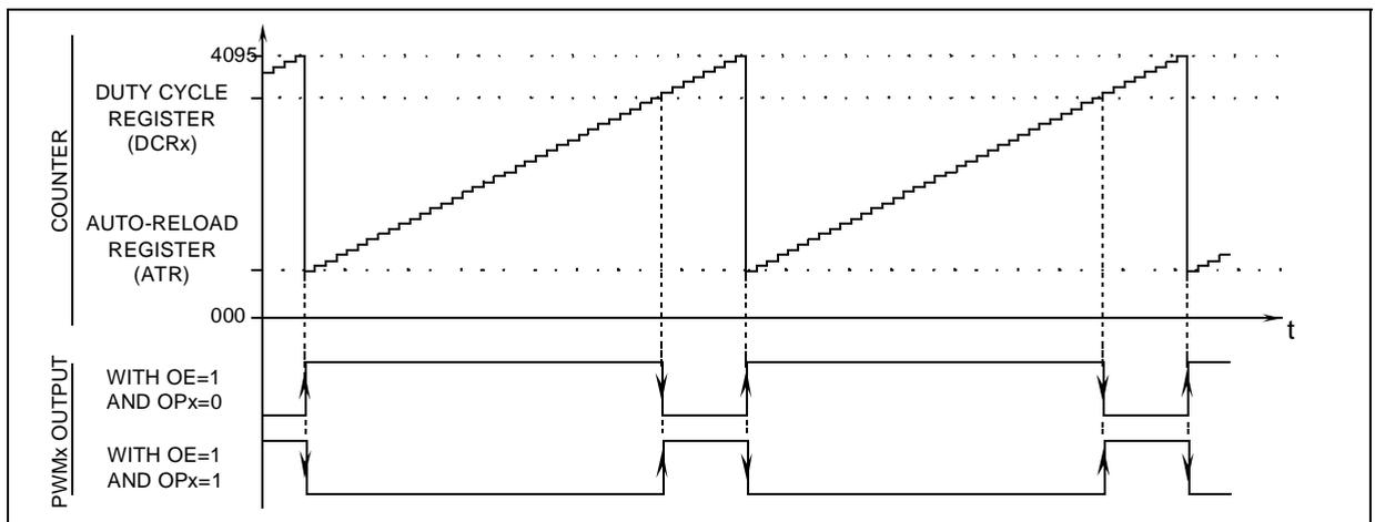
contents of the corresponding DCRx register must be greater than the contents of the ATR register.
