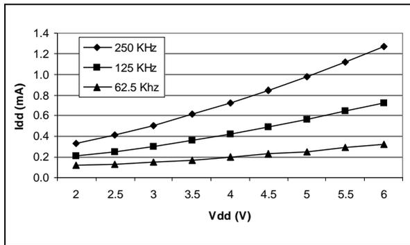
Figure 64. Typical  $I_{DD}$  in AWUFH mode at  $T_A=25^\circ\text{C}$
