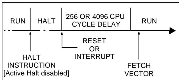
Figure 25. HALT Mode Flow-chart
