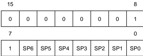
The Stack Pointer is a 16-bit register which is always pointing to the next free location in the stack. It is then decremented after data has been pushed onto the stack and incremented before data is popped from the stack (see Figure 11).
