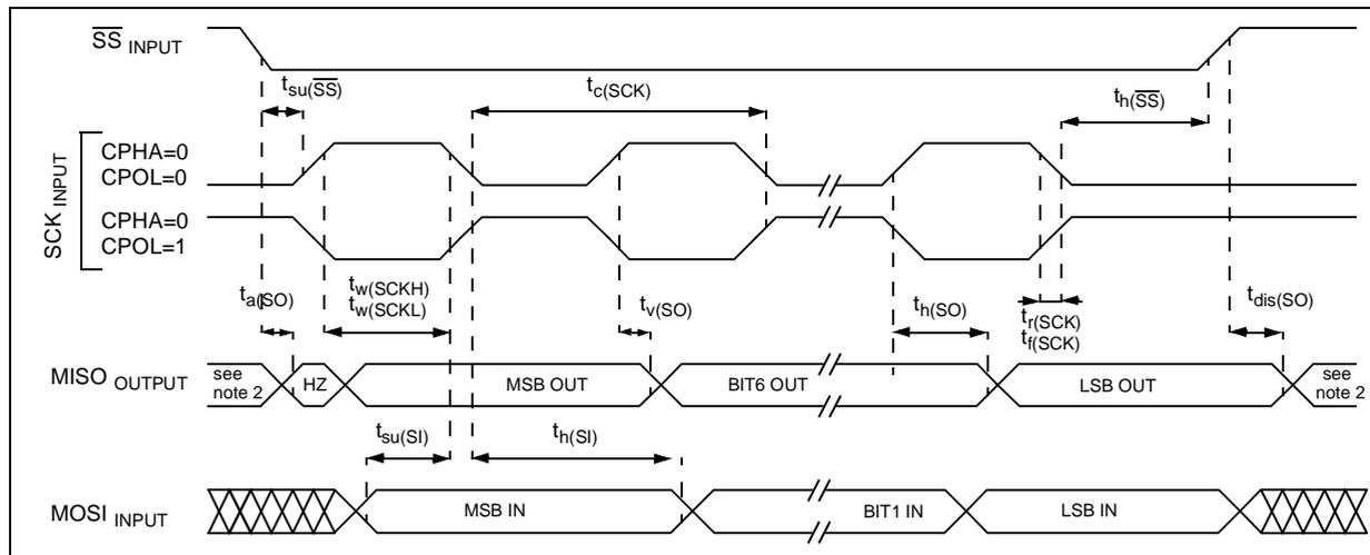
Figure 91. SPI Master Timing Diagram <sup>1)</sup>
