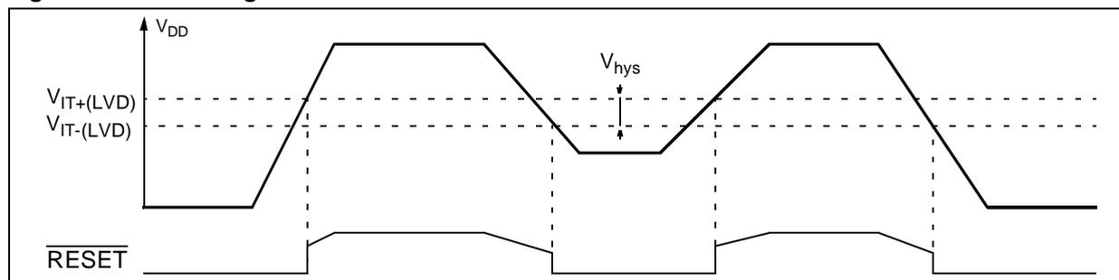
The voltage threshold can be configured by option byte to be low, medium or high.
