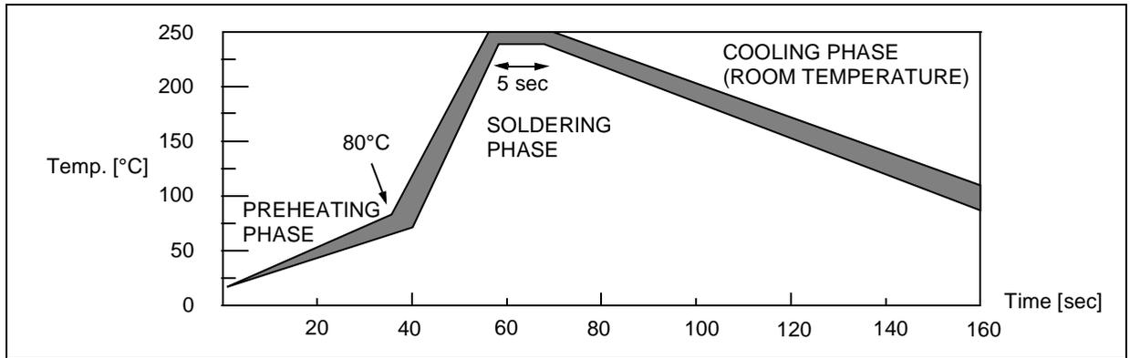
Figure 97. Recommended Reflow Soldering Oven Profile (MID JEDEC)
