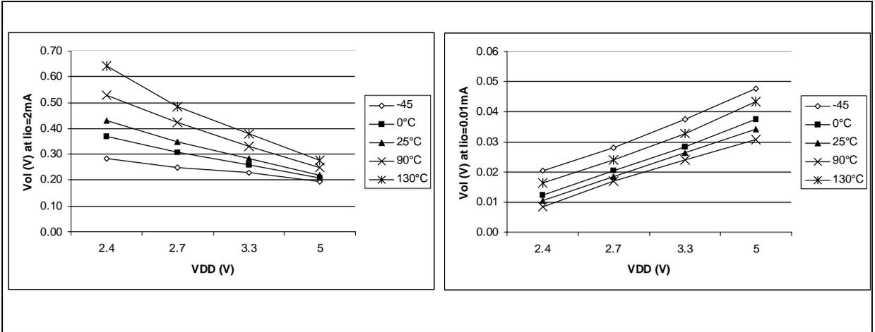
Figure 86. Typical  $V_{OL}$  vs.  $V_{DD}$  (high-sink I/Os)
