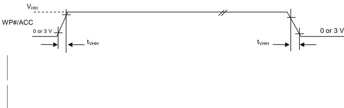
**Figure 12. Sector Group Protect and Chip Unprotect Timing Diagram**
