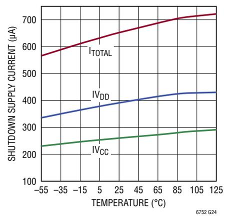
**TYPICAL PERFORMANCE CHARACTERISTICS AC**  $V_{CC} = V_{DD} = 2.5V$ ,  $C_{LOAD} = 5pF$ ,
