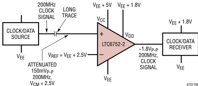
Figure 8. High Speed Clock Restoration/Level Translation/Level Shifting Circuit
