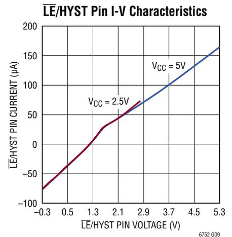
**TYPICAL PERFORMANCE CHARACTERISTICS DC**  $V_{CC} = V_{DD} = 2.5V$ ,  $C_{LOAD} = 5pF$ ,
