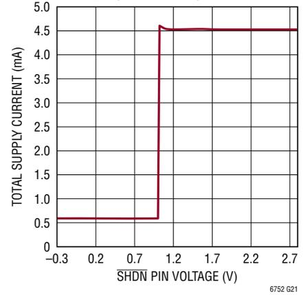
**Total Supply Current vs SHDN Pin Voltage (LTC6752-3)**
