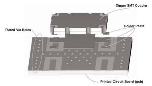
Figure 4: Mounting Features Example
