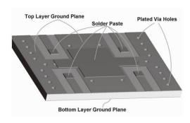
Figure 2: Solder Paste Application
