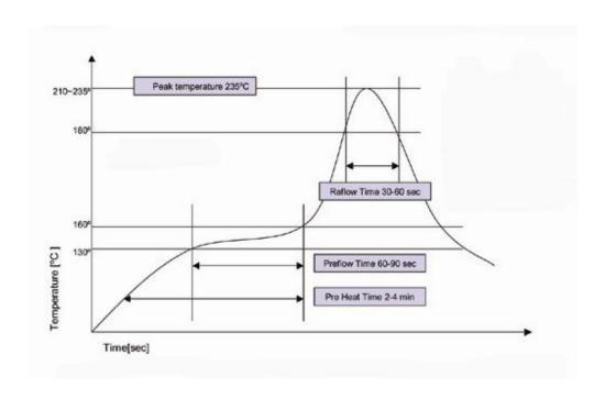
Figure 5 - Low Temperature Solder Reflow Thermal Profile
