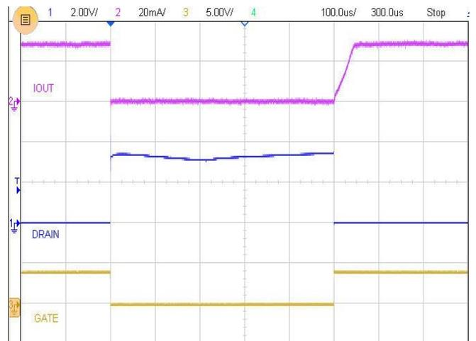
**Figure 8 Minimum Off Pulse Width ( $t_{OFF\_MIN}$ )**
