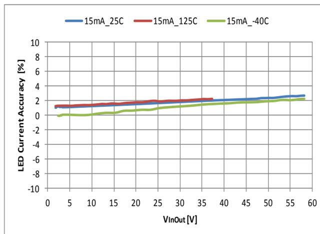
**Figure 17 LED Current Accuracy (%) vs. VinOut across Temperature**
