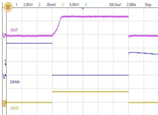
**Figure 7 Minimum On Pulse Width ( $t_{ON\_MIN}$ )**
