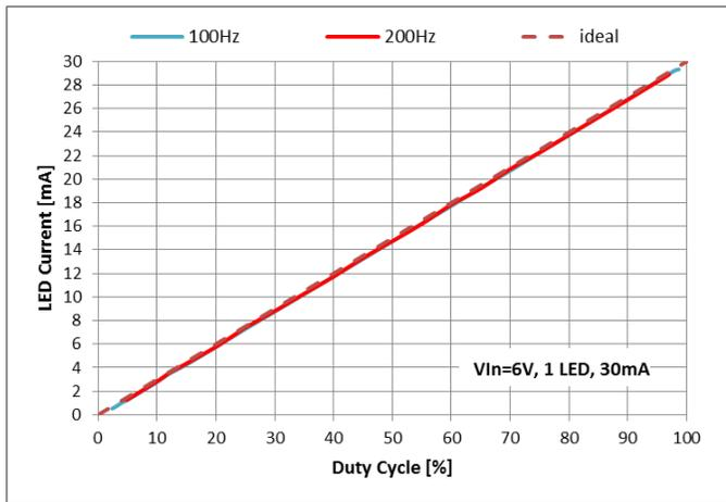
**Figure 5 PWM Dimming 30mA vs. Duty Cycle**
