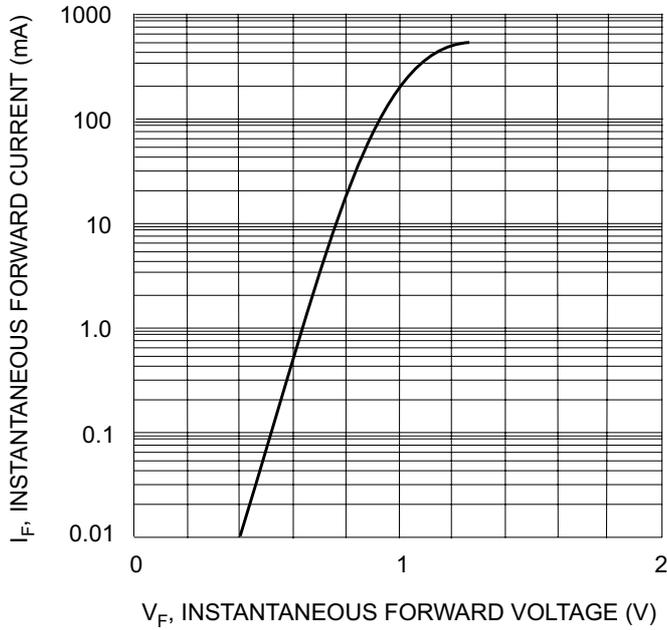
Fig. 1 Forward Characteristics
