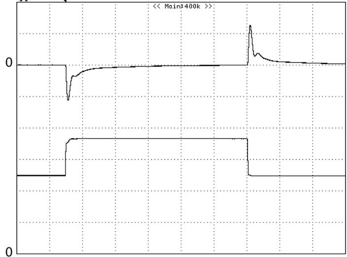
**Figure 9:** Output voltage response to step-change in load current (75%-50%-75% of  $I_o$ , max;  $di/dt = 2.5A/\mu s$ ). Load cap:  $470\mu F$ ,  $35m\Omega$  ESR solid electrolytic capacitor and  $1\mu F$  ceramic capacitor. Top Trace:  $V_{out}$  (50mV/div, 200us/div), Bottom Trace:  $I_{out}$  (5A/div). Scope measurement should be made using a BNC cable (length shorter than 20 inches). Position the load between 51 mm to 76 mm (2 inches to 3 inches) from the module
